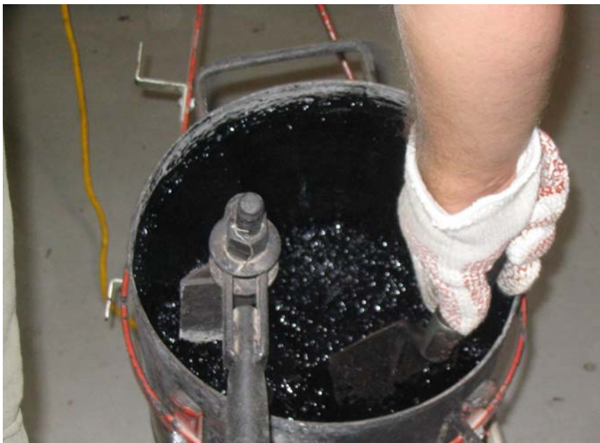
Figure 3.5. Warm Mix Asphalt in Bucket Mixer.
