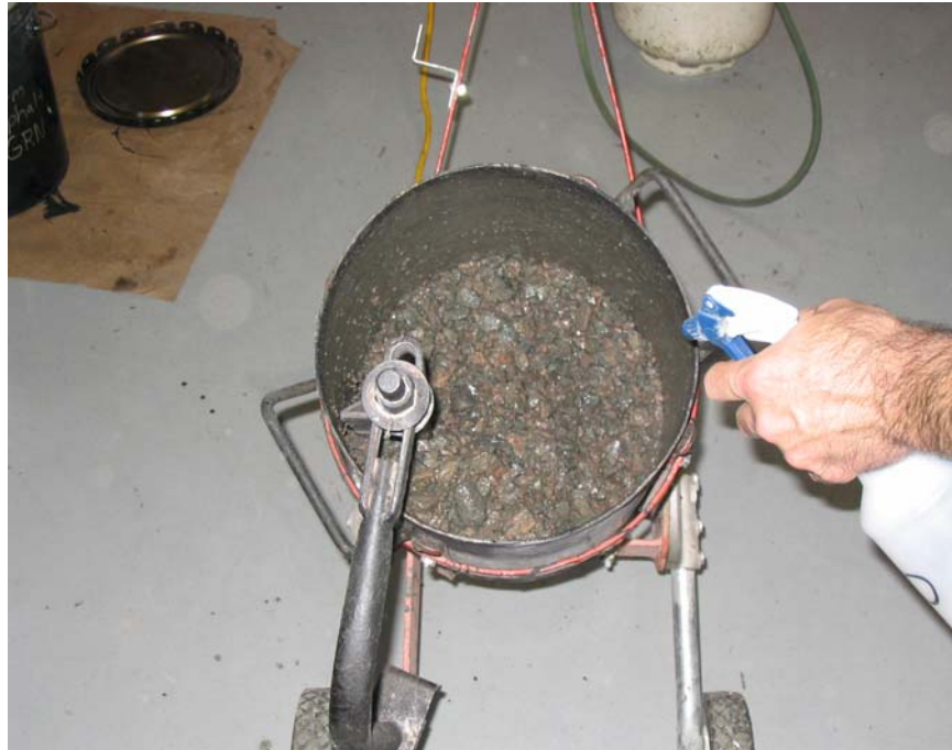
Figure 3.3. Introduction of Moisture to Aggregate for TSR Samples.
