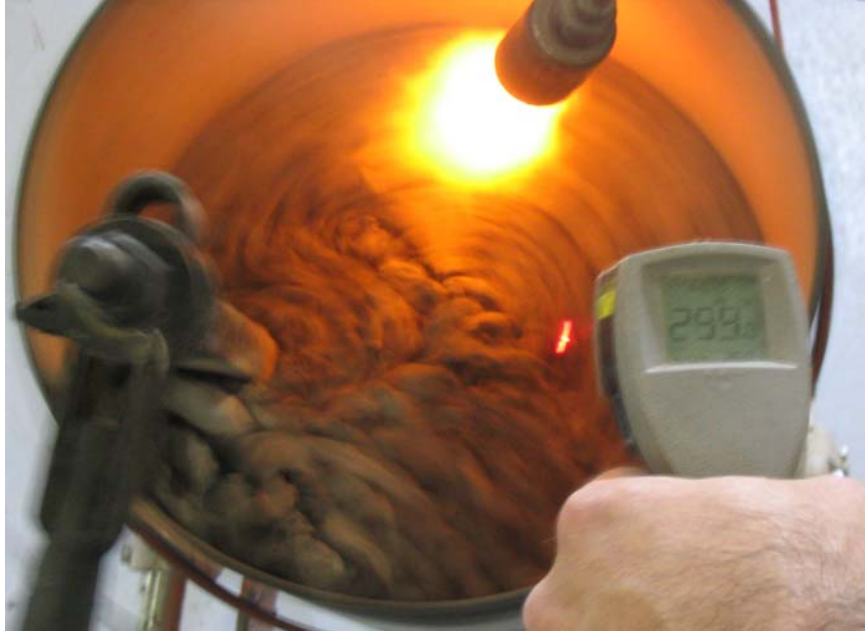
Figure 3.4. Heating of Wet Aggregate to Mixing Temperature.
