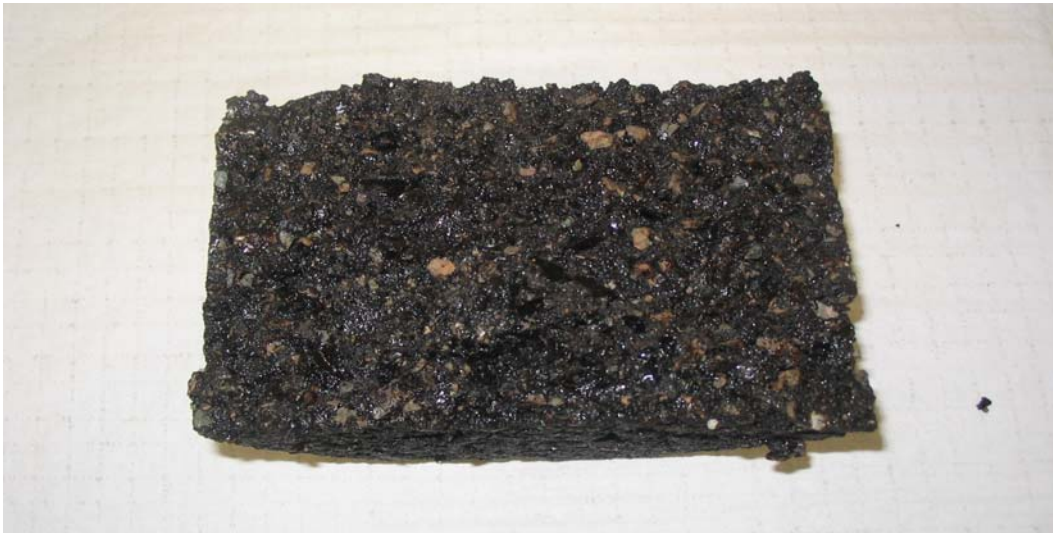
Figure 4.13. Example of Adhesive Stripping Failure – Granite.
