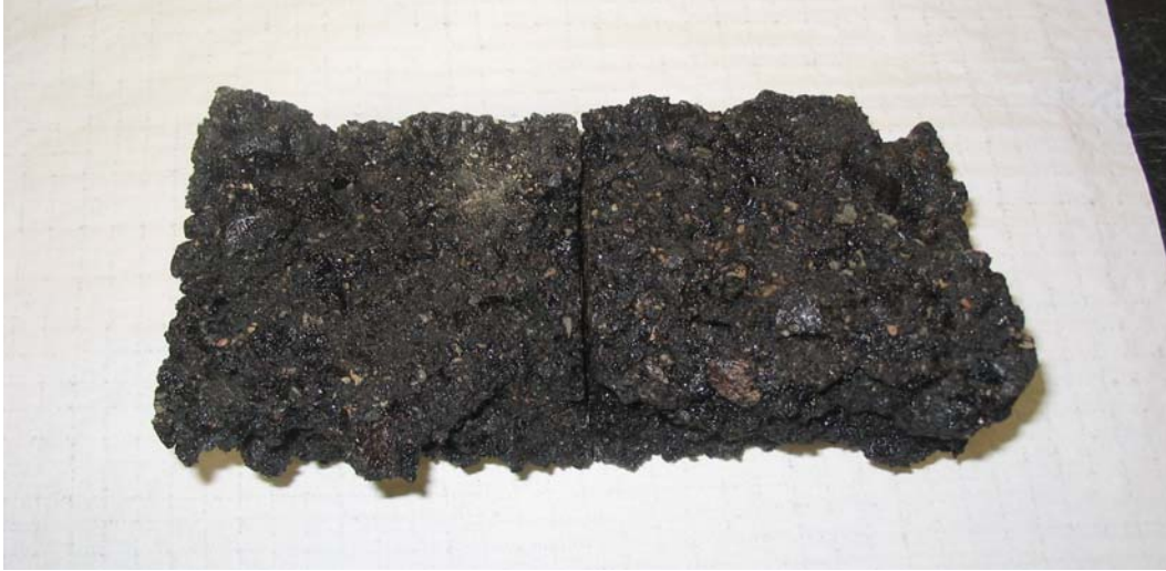
Figure 4.12. Example of Cohesive Stripping Failure – Granite.
