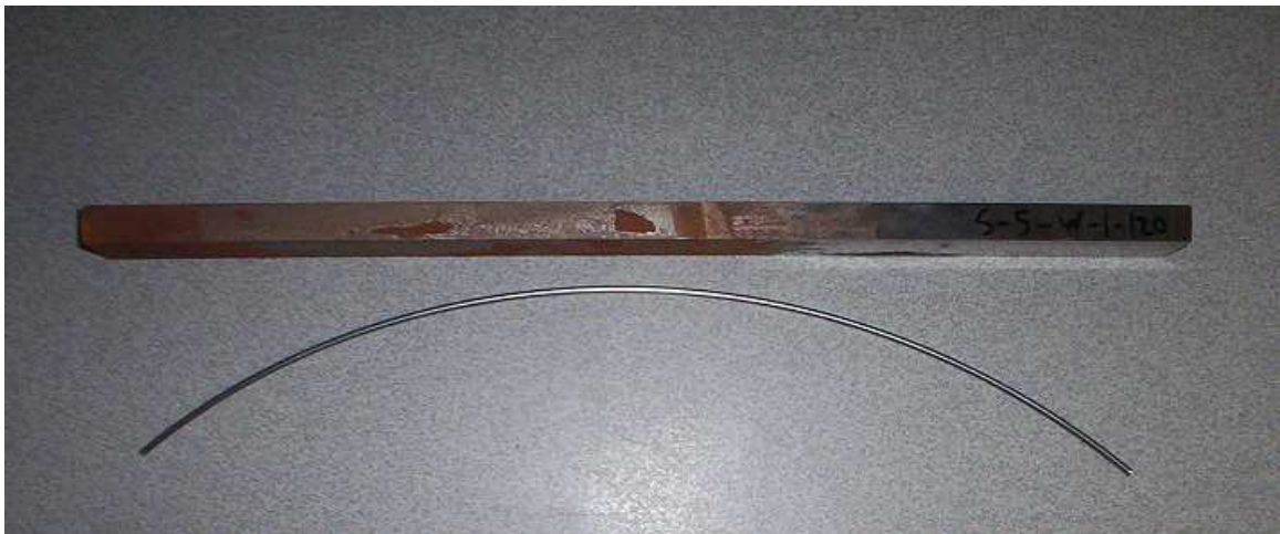
Figure 5.7 Comparison of steel (top) and nitinol (bottom) after five days in seawater
