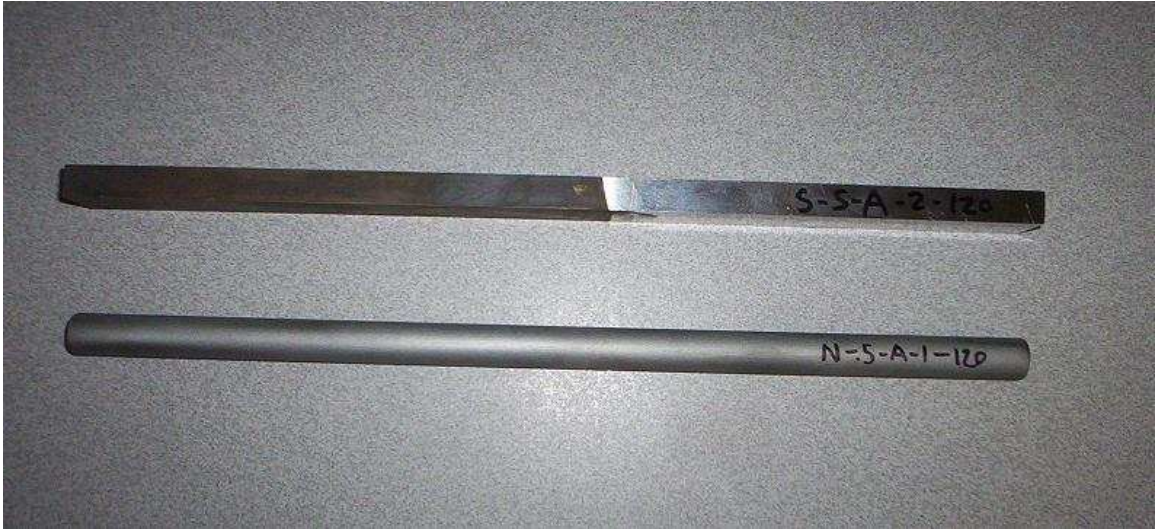
Figure 5.3 Comparison of steel (top) and nitinol (bottom) after five days in sulfuric acid
