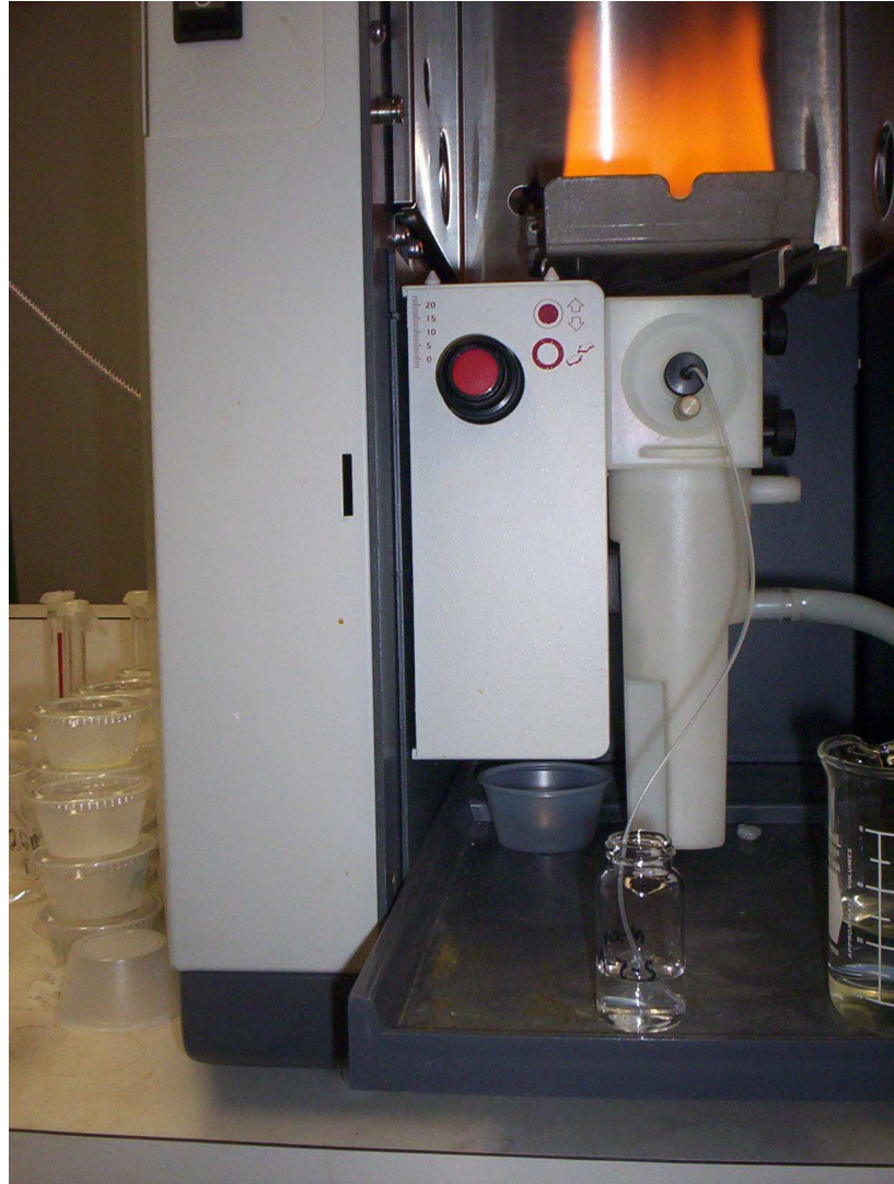
Figure 4.7 Measuring nickel concentration with the AAS
