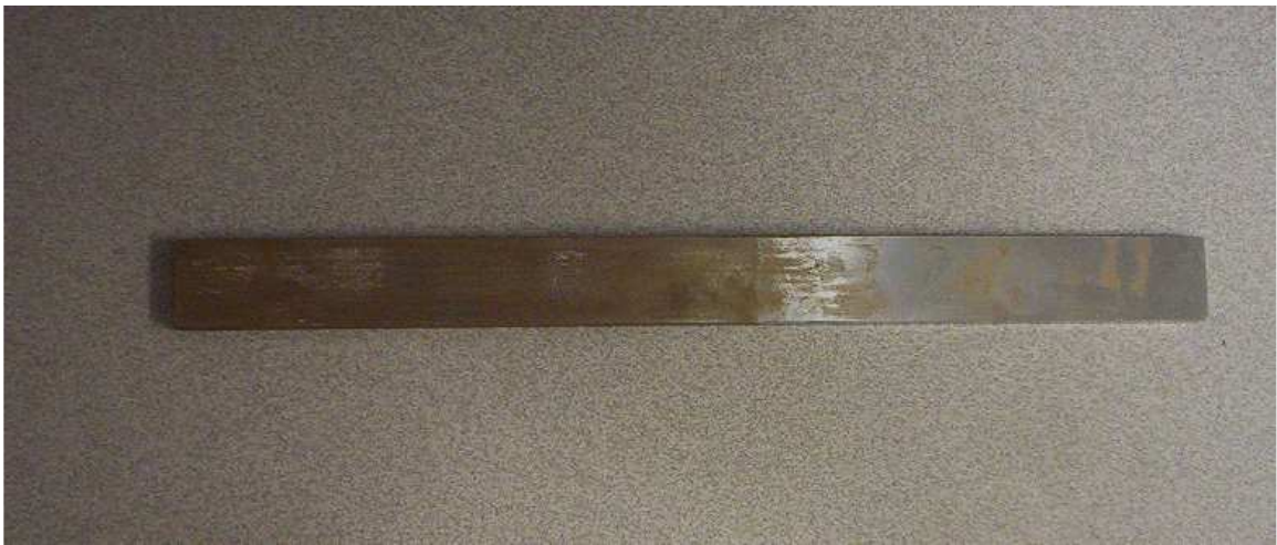
Figure 5.6 Steel specimen after less than twenty minutes in seawater
