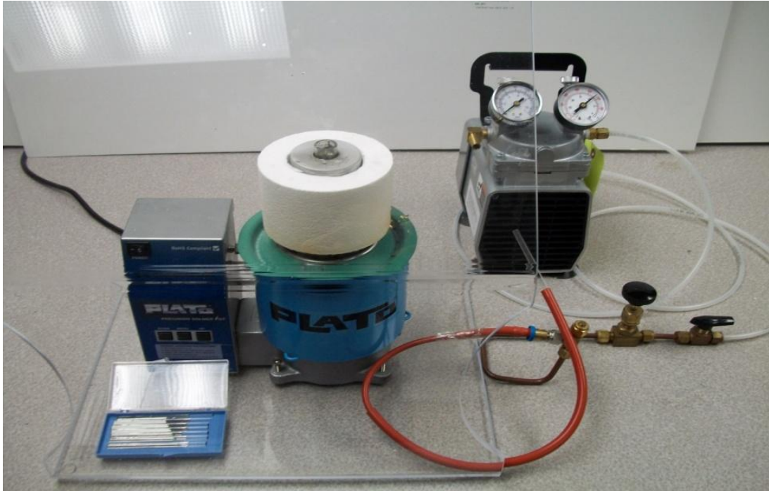
Figure 41: Setup for Innolot tensile specimen preparation [Lall et. al. 2012]
