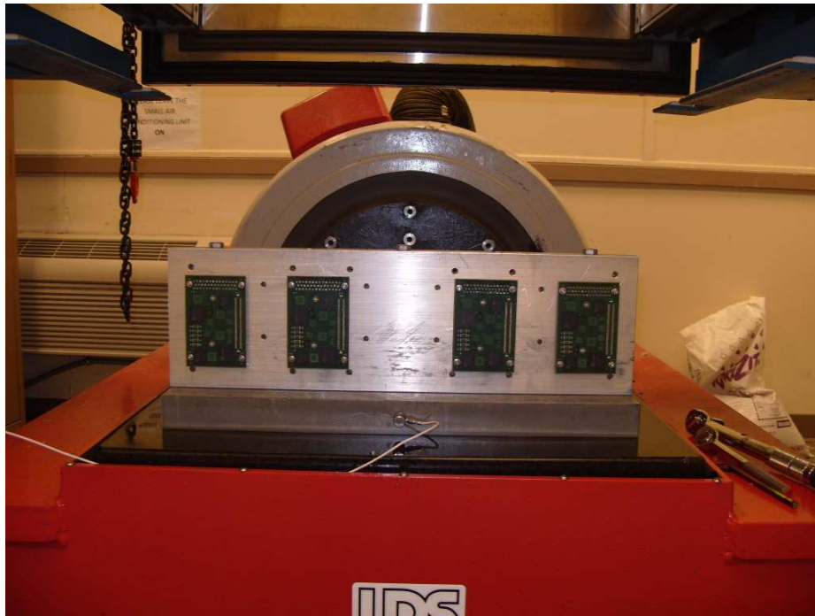
Figure 5.2 Fixture capable of testing 8TV7 boards
