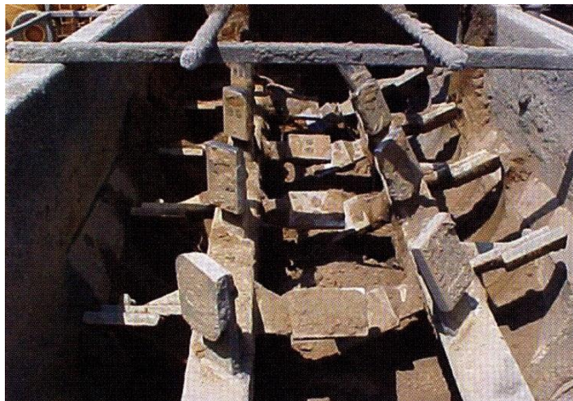
Figure 2.23: Twin-shaft pug-mill mixing chamber (Halsted et al. 2006)
