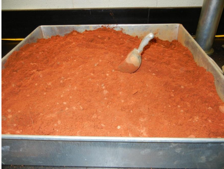
Figure 3.11: Soil-cement in pan
