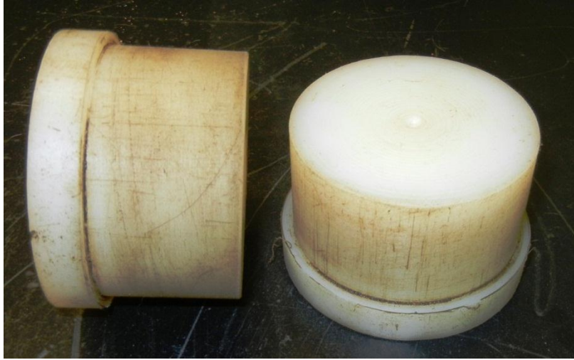
Figure 3.7: UHMW Mold Plugs
