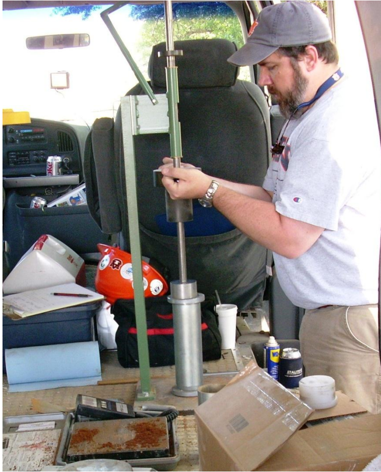
Figure 3.1: Sample compaction at field location
