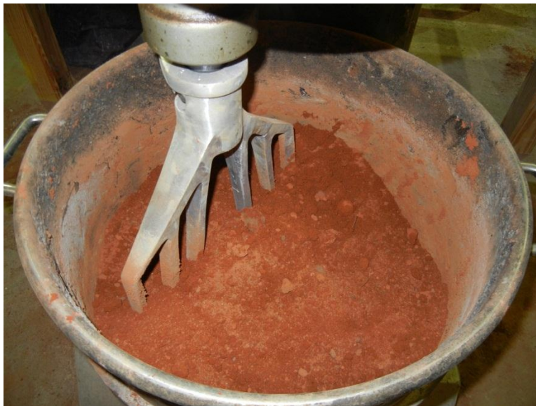
Figure 3.10: Soil and water being mixed in mixer bowl
