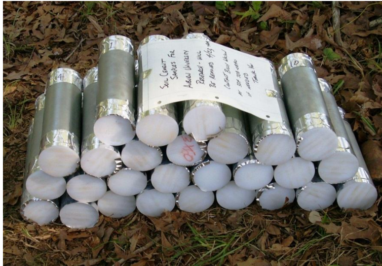
Figure 3.19: Molded specimens stored during initial curing
