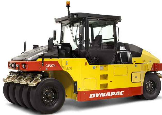
Figure 2.26: Multiple-wheel, rubber-tire roller used to compact soil-cement base (Dynapac 2012)
