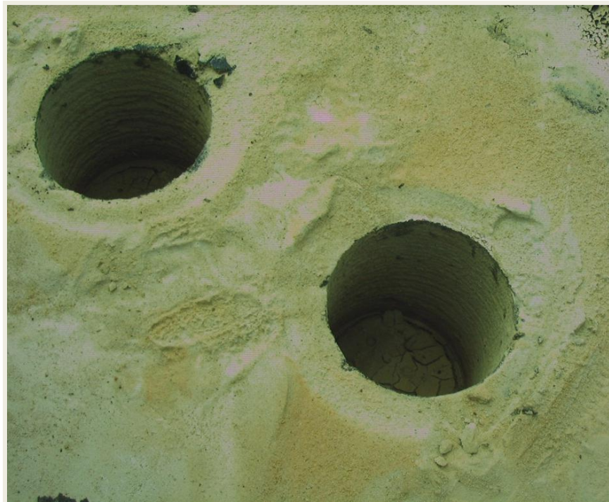
Figure 1.3: Core holes in soil-cement base
