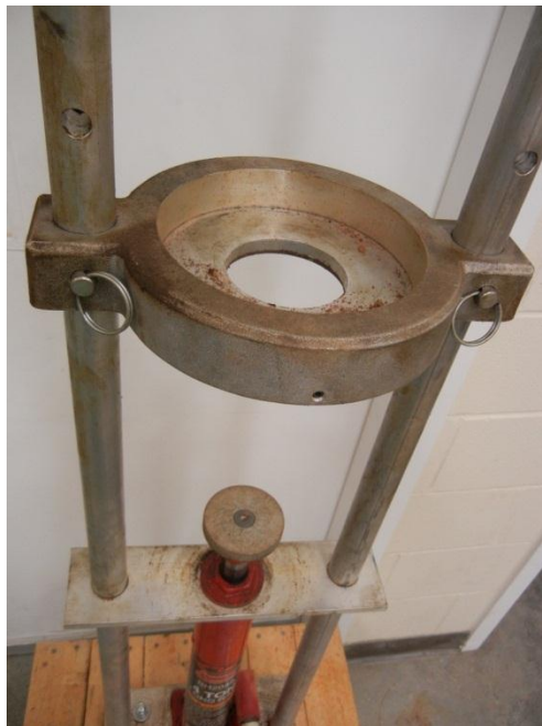
Figure 3.23: Close up of vertical hand-jack used for sample de-molding
