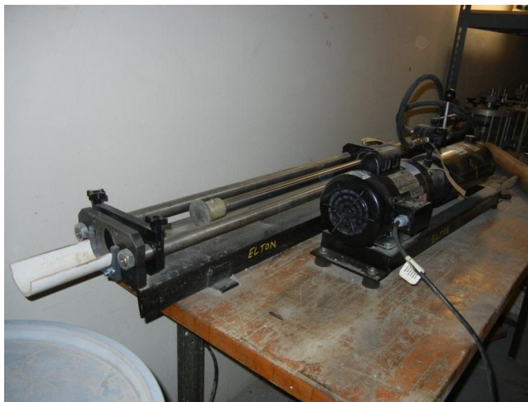
Figure 3.20: Horizontally mounted hydraulic extruder
