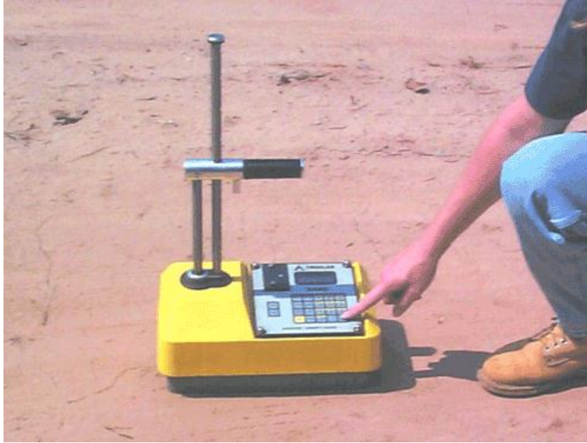
Figure 2.28: Nuclear Density Measurement (FHWA 2011)
