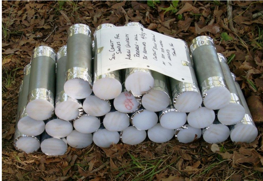
Figure 5.4: Molded specimens during initial curing period
