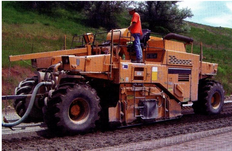
Figure 2.20: Single-shaft traveling mixer used in mixed-in-place construction (Halsted et al. 2006)
