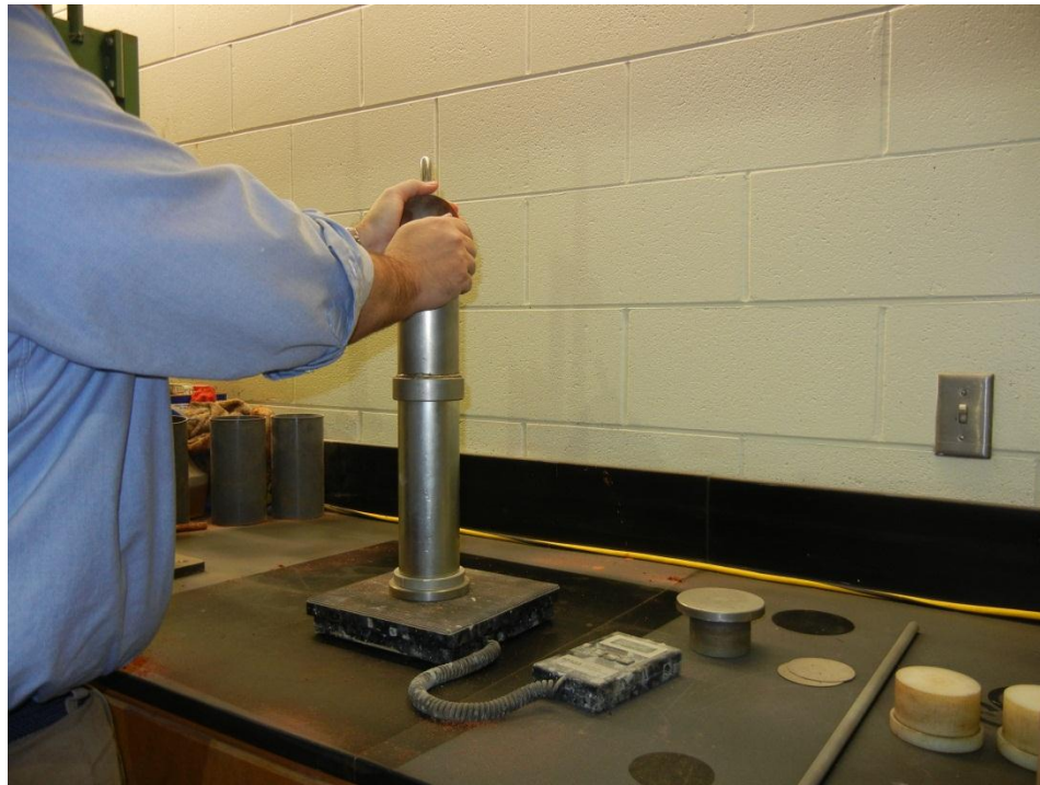
Figure 3.15: Soil-cement mixture being placed into the mold
