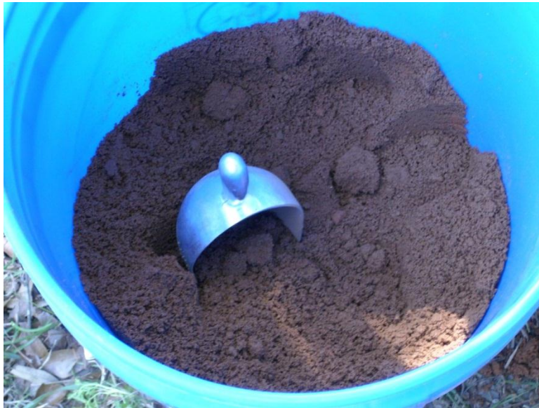
Figure 3.4: Composite sample of soil-cement mixture in 5-gallon bucket
