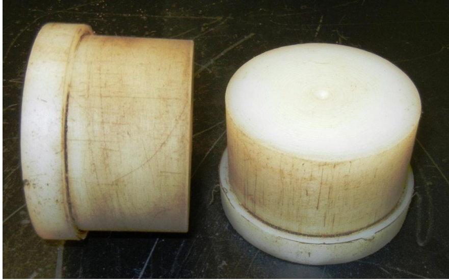
Figure 5.3: UMHW Mold Plugs
