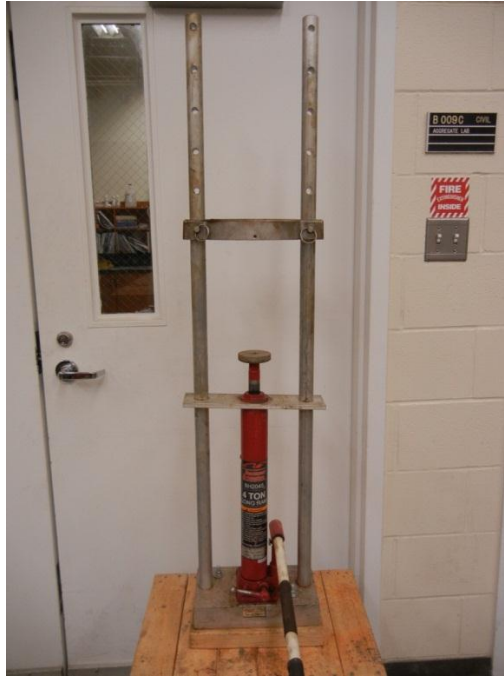
Figure 3.22: Vertical hand-jack used for sample de-molding
