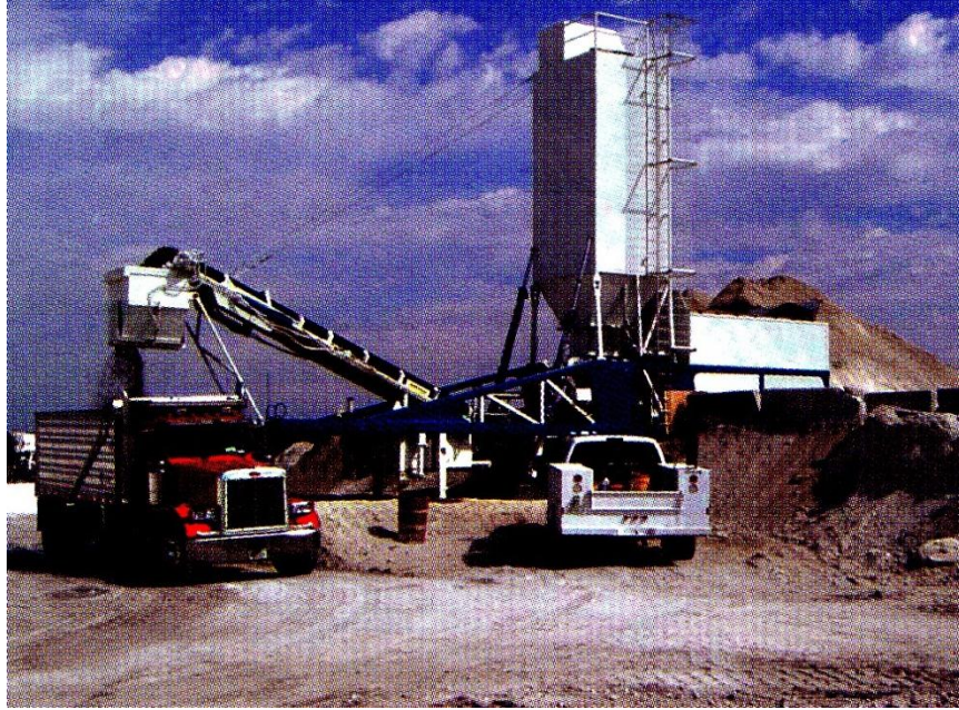
Figure 1.2: Typical central mixing plant for soil cement (Halsted et al. 2006)
