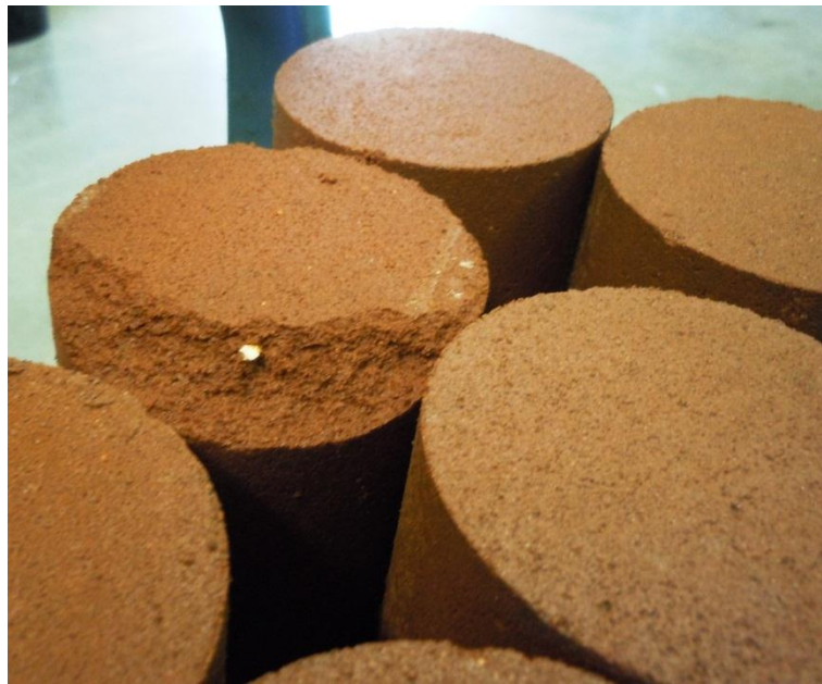
Figure 3.21: Edge cracking from horizontally mounted, hydraulic extruder
