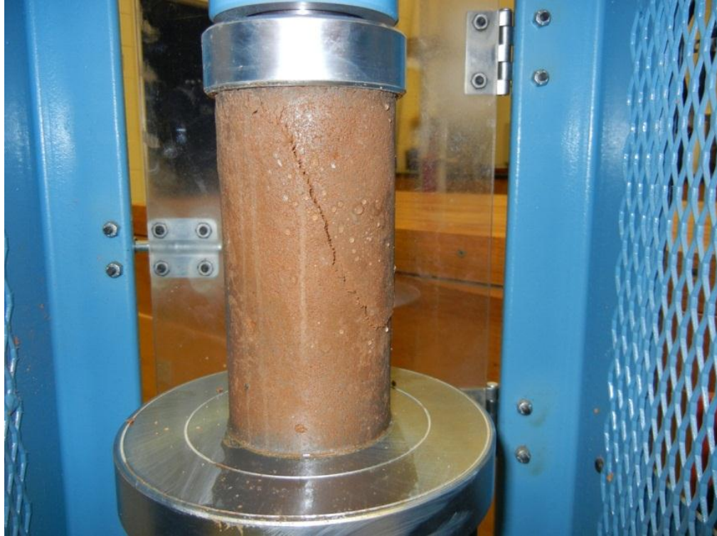
Figure 3.26: Sample after failure
