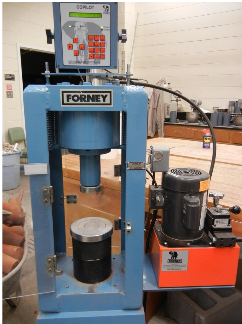
Figure 3.24: Compression testing machine
