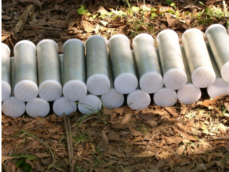
Figure 3.18: Molded specimens before foil tape addition
