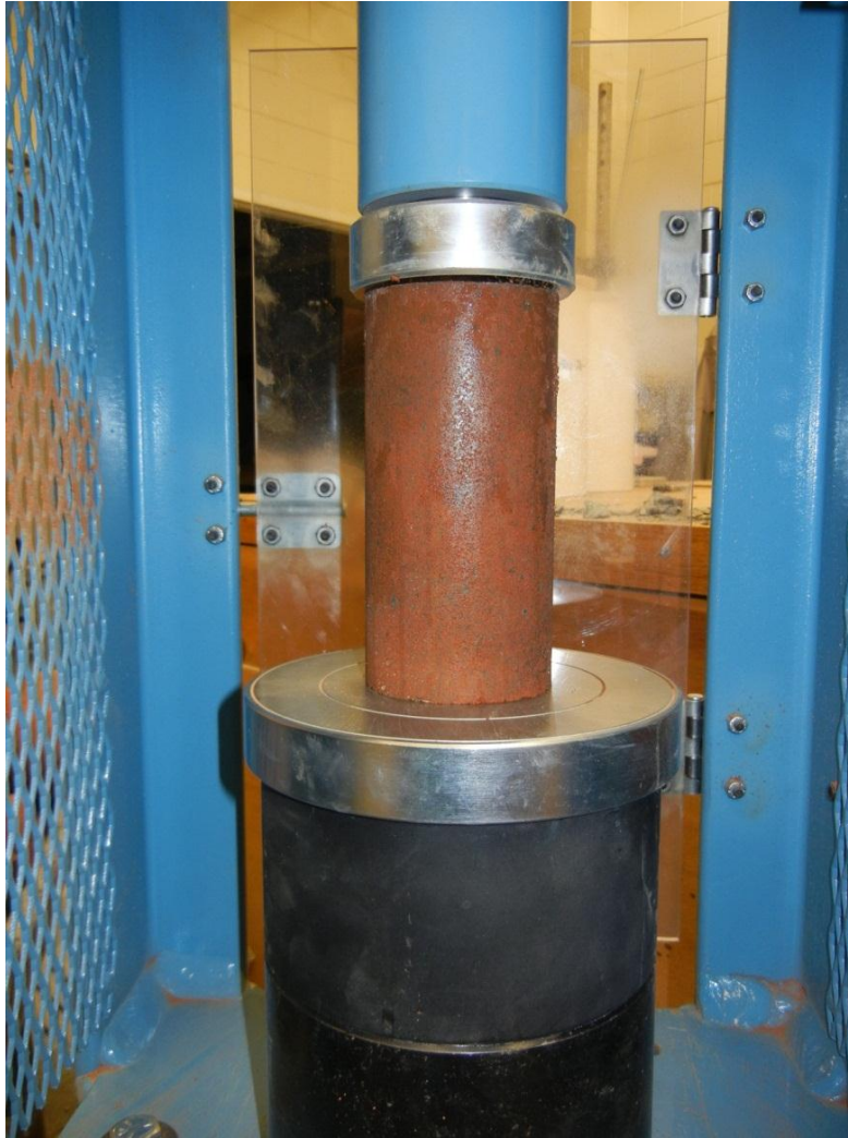
Figure 3.25: Sample loaded into compression testing machine
