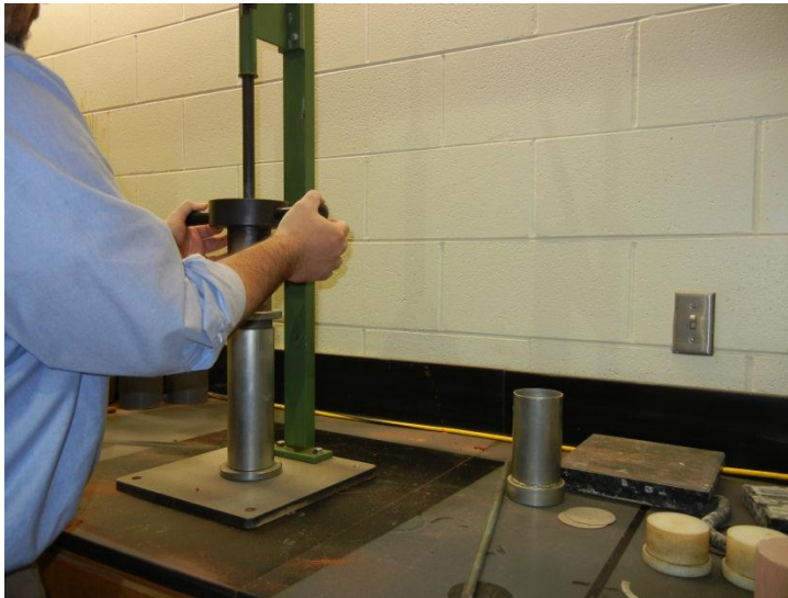
Figure 3.17: Soil-cement mixture being compacted until refusal
