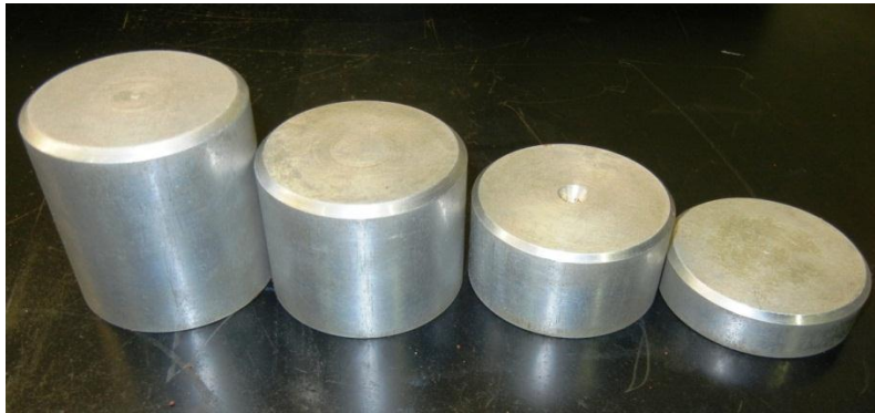
Figure 3.2: Aluminum spacer disks for the L/D study
