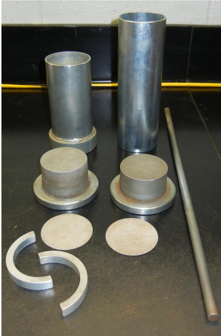
Figure 3.13: Soil-cement cylinder mold
