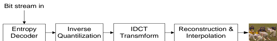
Figure 1.8: Block diagram of a typical video decoder.
