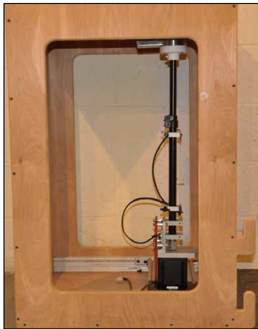
Figure 20. Pressure application mechanism under seat pan.
