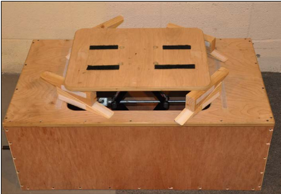
Figure 22. Local pressure application apparatus foot rest.
