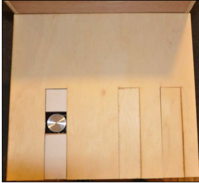
Figure 23. Seat pan prepared for posterior thigh pressure application.
