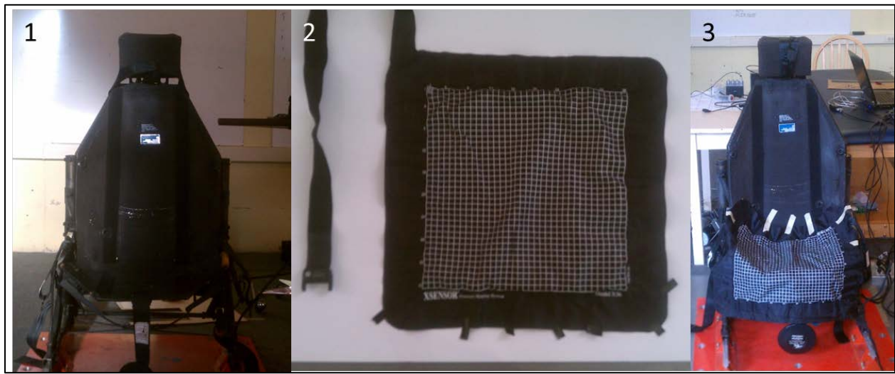
Figure 19. Seat interface pressure mapping system. 1: Black Hawk seat without mapping system; 2: Pressure mapping system; 3: Pilot's seat and mapping system integrated.
