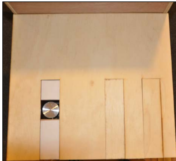
Figure 33. Local pressure application head integrated into seat pan.
