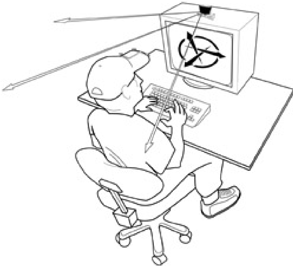
Figure 3.4: TrackIR4 Reading Position and Orientation via TrackClip[8]
