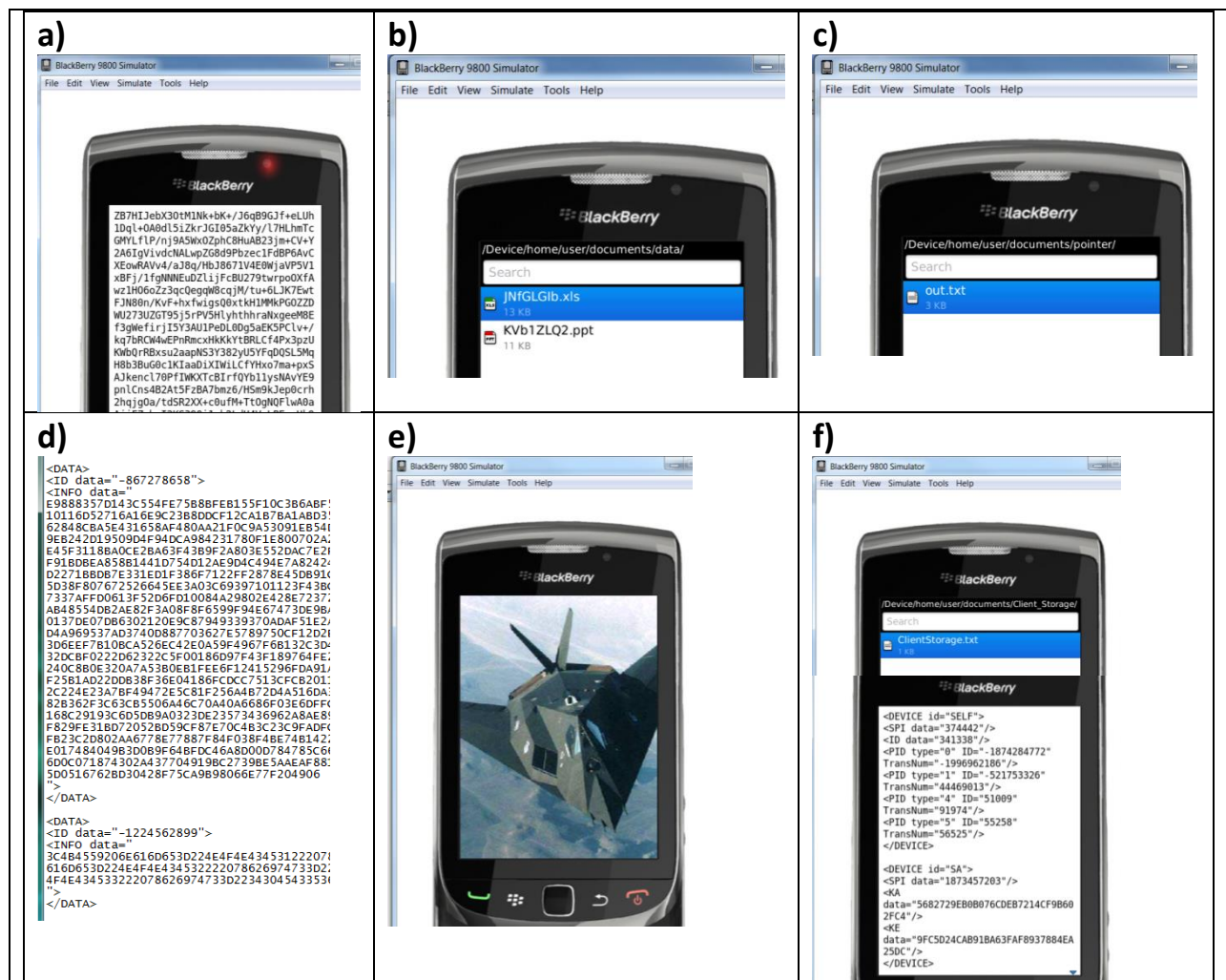
Fig. 60. BlackBerry implementation of IDACS encryption and distributed storage. (a) file ciphertext with Xslices removed is (b) divided and stored in multiple data files. (c) Names of data files are encrypted and stored in a pointer file. (d) Xslices and Xbits are stored on IDACS Database as pure data; no information saved on Database indicating the identity of this data. (e) Correctly reassembling all distributed and mutated pieces results in correct file decryption. (f) Distributed storage between Client and User Badge is simulated using separate text files.
