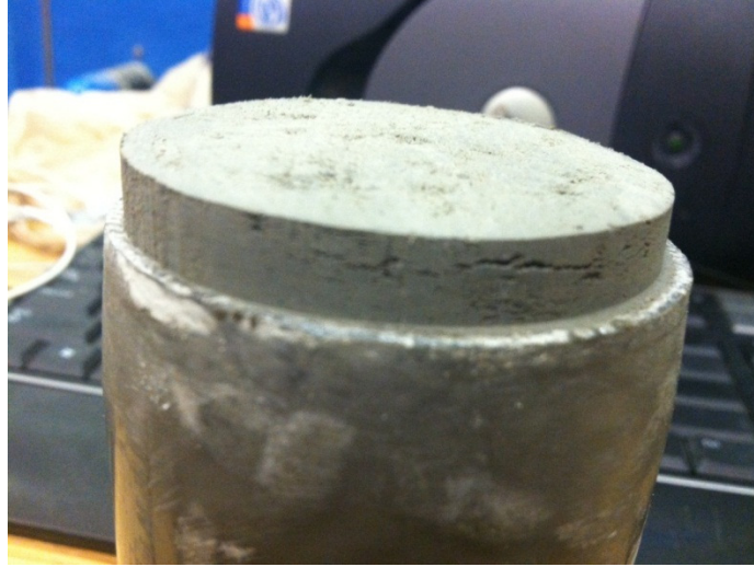
Figure 4-20. Prairie Bluff Chalk Formation Cracking Example 1
