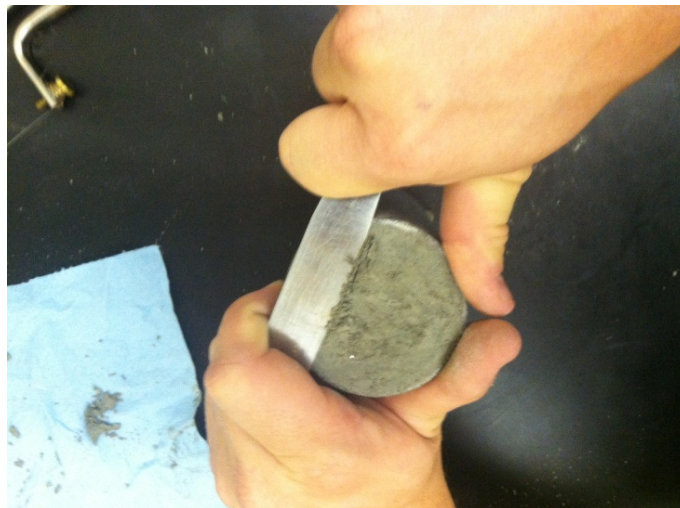
Figure 3-14. Cutting and Cleaning Surface of Sample
