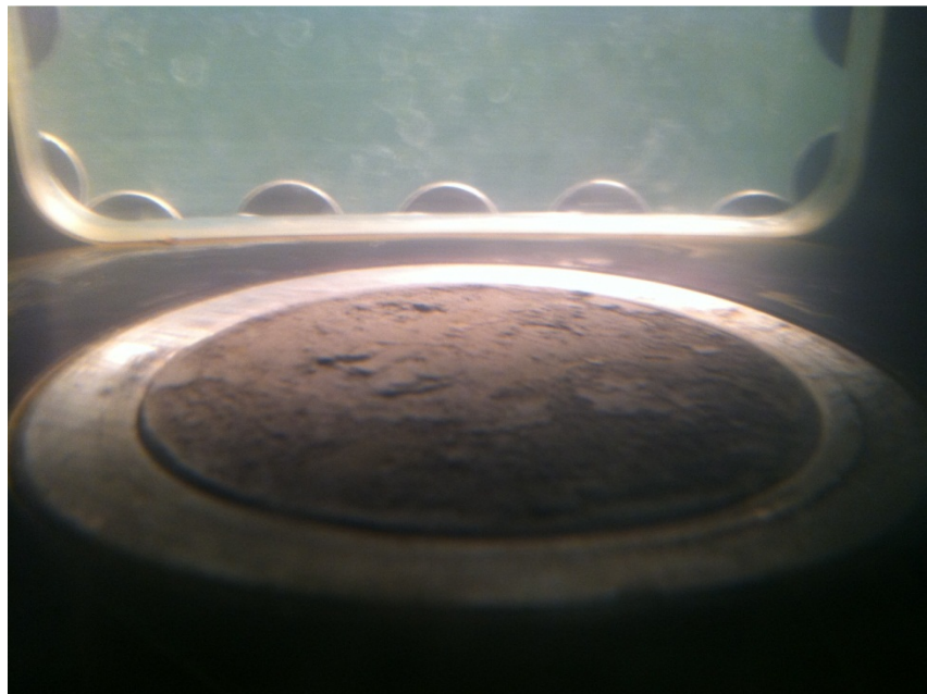
Figure 3-16. Soil Sample in EFA Level with Base of Flume
