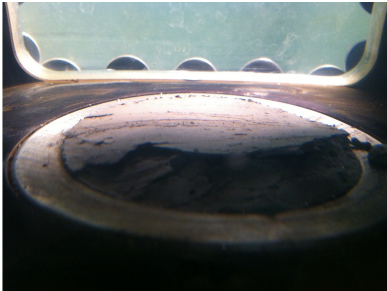
Figure 4-8. “Yazoo Clay 18.5_1” Test Failure Wedge
