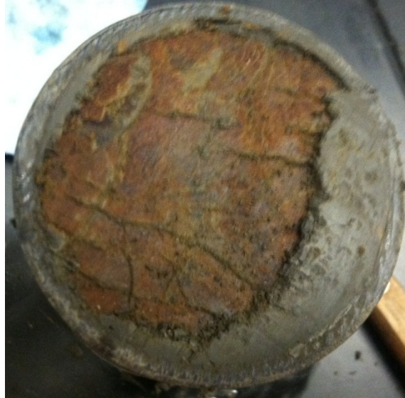
Figure 4-23. Porter’s Creek Clay Formation Scoured along Weathered Planes
