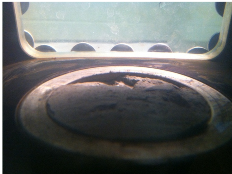
Figure 4-12. “Yazoo Clay 18.5_9” Test Scoured Area from Front
