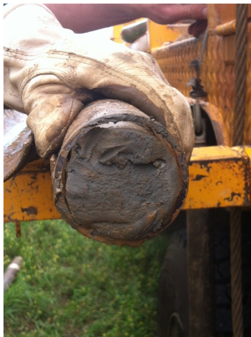
Figure 4-2. Bucatunna Clay Sample Smaller Radially than Sample Tube
