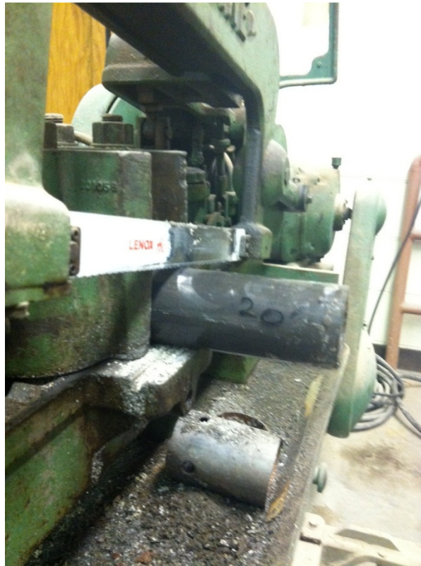
Figure 3-12. Automatically Advancing Hacksaw Cutting Sample Tube
