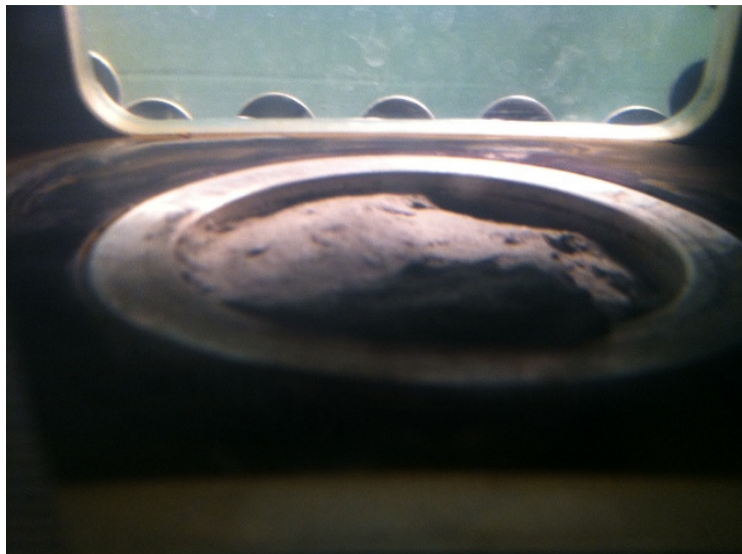
Figure 4-10. “Yazoo Clay 18.5_2” Test After Failure
