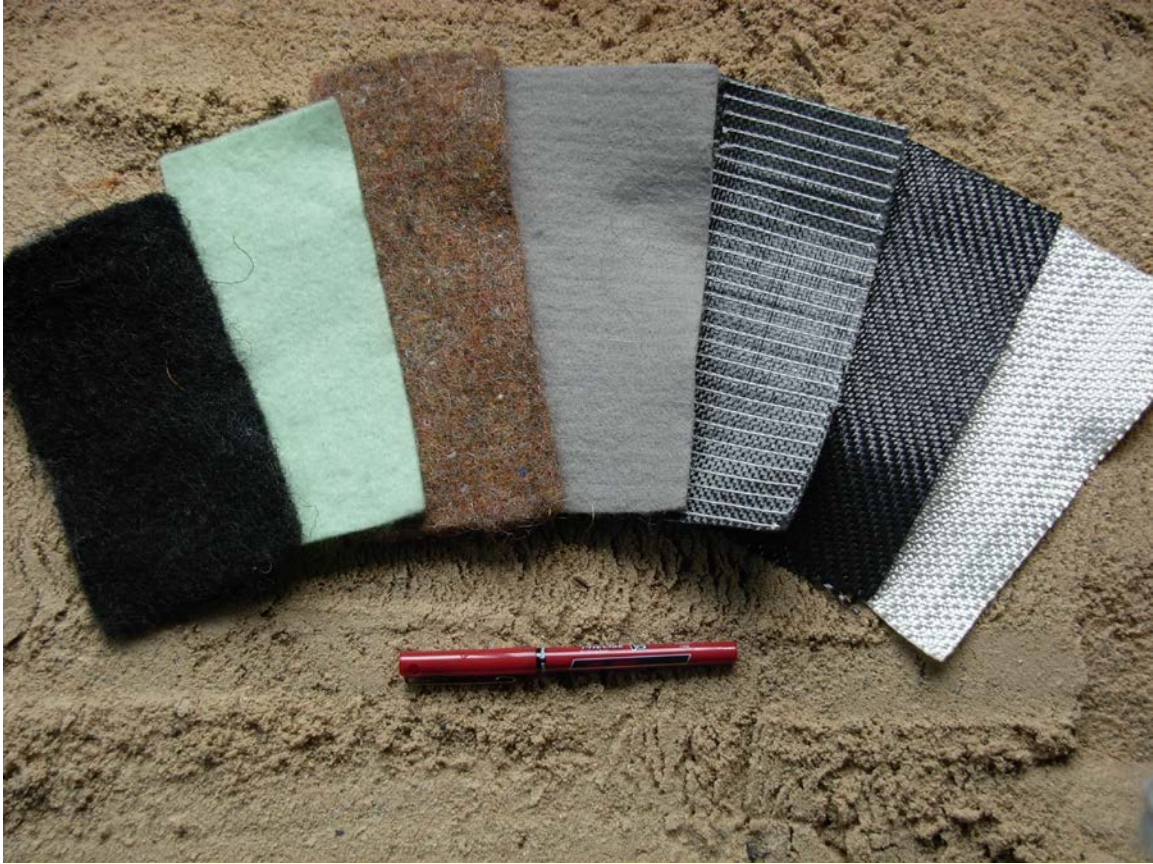
Figure 1.1: Examples of geotextiles, showing four nonwoven samples (left) and three woven samples (right). Source: Wikipedia Commons 2008.
