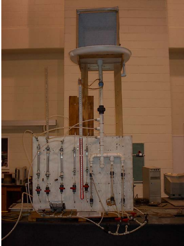
Figure 4.2: Photograph of the bubble point apparatus. Source: Elton et al. 2007.
