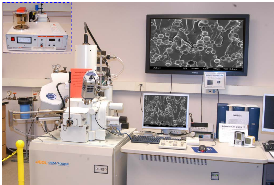
Fig. 3.11: Photograph of Scanning Electron Microscope (Model: JEOL JSM-7000F) used to study fracture surface morphologies of particulate polymer composites. The top left inset shows the photograph of a gold sputtering unit (Model: PELCO SC-6) used for SEM sample preparation.
