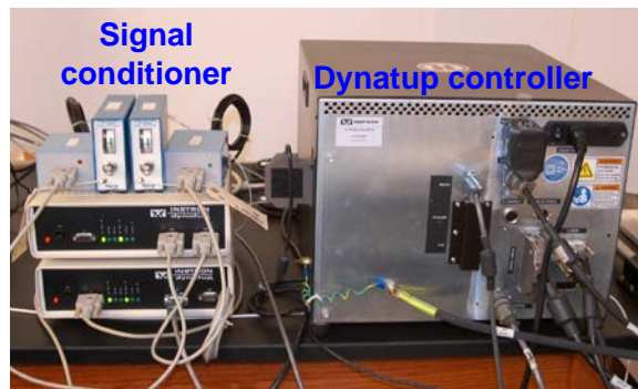
Fig. 3.3: Photographs of the experimental setup used for dynamic fracture study.
