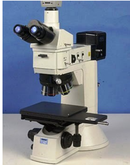
Fig. 3.9: Photograph of Nikon Eclipse L150 optical microscope used for checking particle distribution in micron-size glass filled PPCs.
