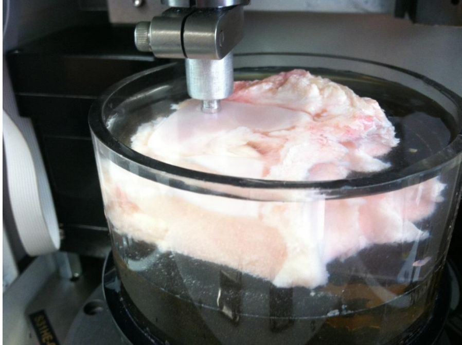
Figure 4.3: UMT-3 performing indentation tests of articular cartilage submerged in saline
