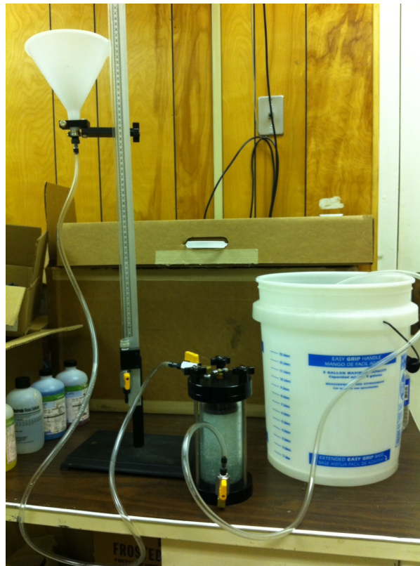
Figure 9. Photograph of permeameter setup. Water flows from a set head through a hydraulic chamber and collects in a bucket.
