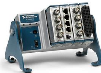
Figure 13: NI Compact DAQ chassis
