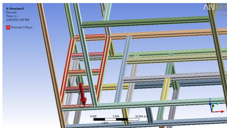
Figure 23: Location of boiling chamber. Red shaded area shows contact area with the extrusion.
