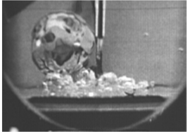
Figure 1.22: Large hovering bubble in R-113; smaller adjacent bubbles near the larger bubble were noticed to migrate towards the larger bubble at high subcooling - Lee and Merte Jr. [43].
