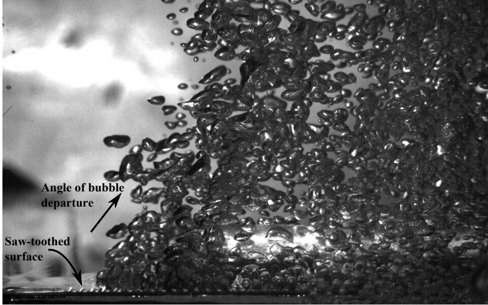
Figure 3.3: Image showing bubble departure from re-entrant cavities at an angle normal to the sloped surface of saw-teeth during saturated pool boiling at a heat flux of q'' = 2.20 \text{ W/cm}^2 .
