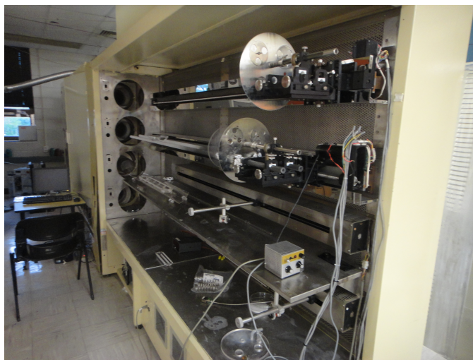
Figure A.7: Oxidation Furnace
