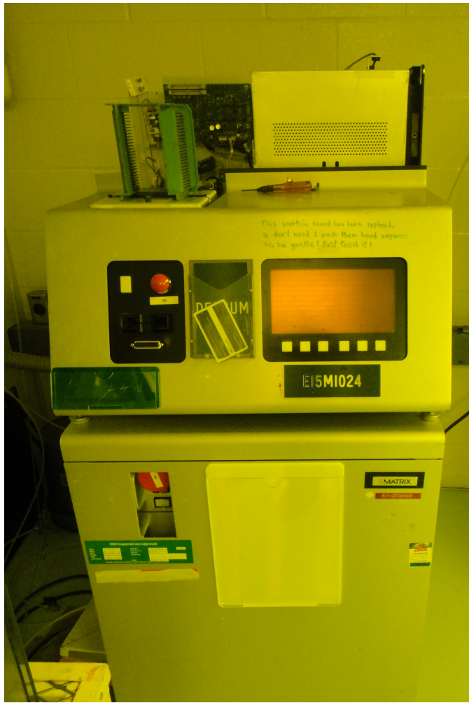
Figure A.5: Matrix O 2 plasma descum
