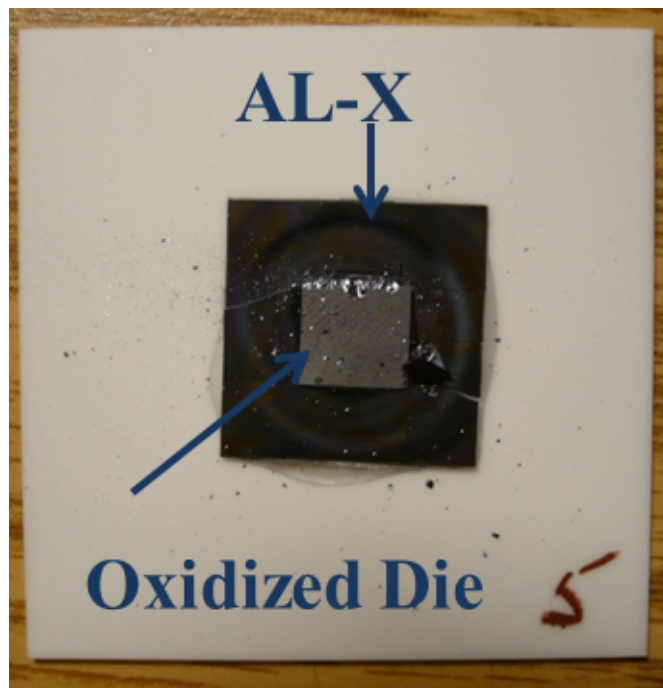
Figure 2.7: Test coupon post-shear mounted on a ceramic carrier.
