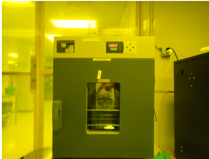
Figure A.2: 135 °C Softbake Oven for AZ-125-NXT-10A
