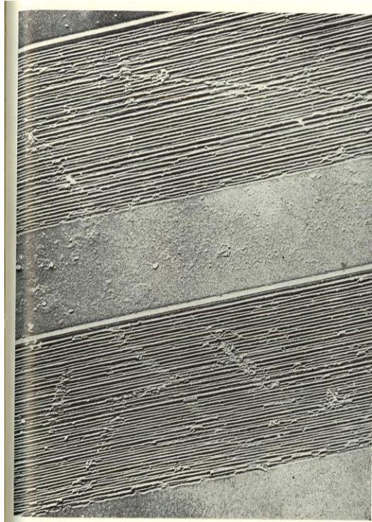
Figure 5. An electron micrograph of a replica of bands nineteen (above) and twenty. These are the finest bands, ruled at an average line spacing of about 0.12 and 0.11 microns respectively (Turner and Bladbury, 1966).
