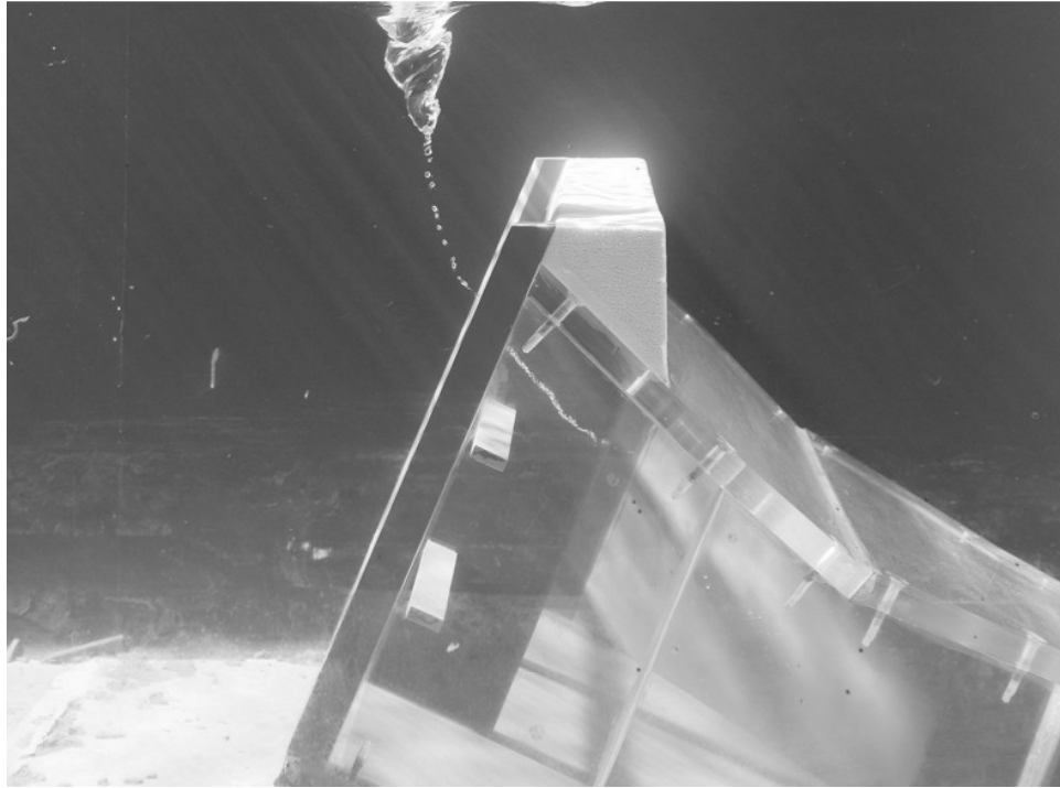
Figure 1.1: Air entraining vortex at intake structure due to insufficient pump submergence [Pinott and Moller(2011)].
