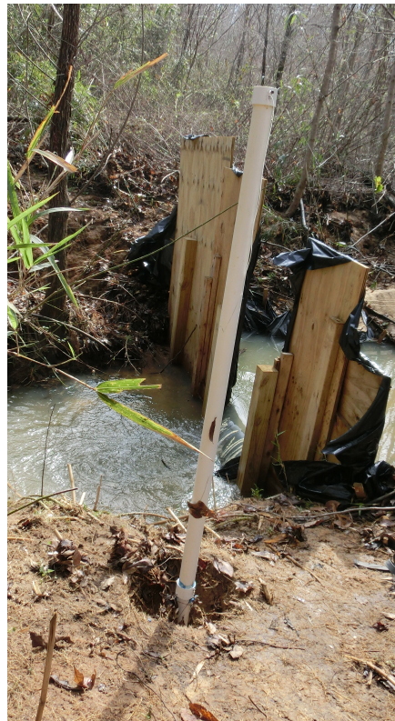
Figure 3.23: Shallow groundwater wells
