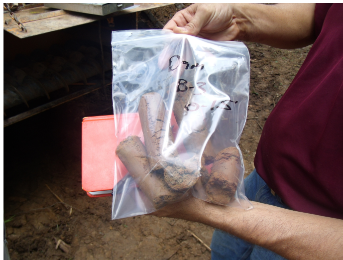
Figure 3.29: Samples taken from the SPT
