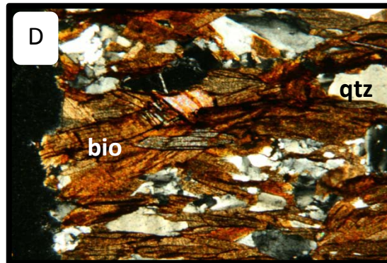
Figure 3. Photographs and photomicrographs of the quartz-biotite schists of the Emuckfaw Group. A. and B. Outcrop views of characteristic ribs. C. Thin section with a 5 mm field of view (in ordinary light). D. Same view as in C., but with crossed polars.
