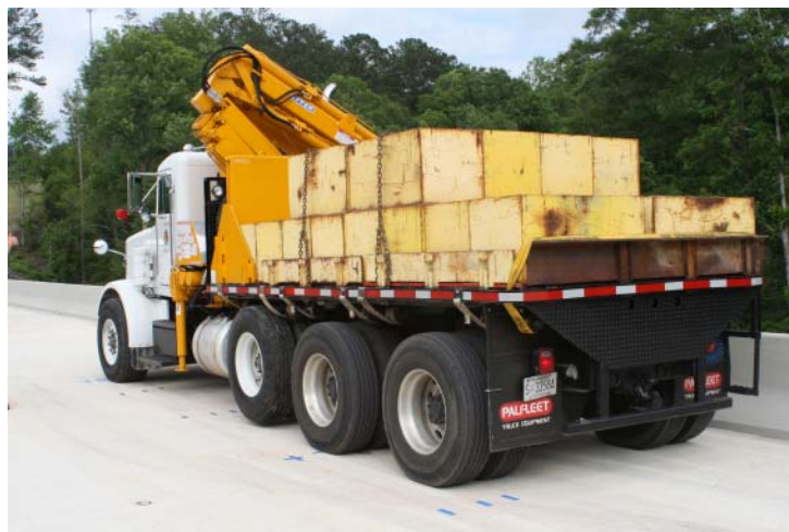
Figure 4.1. ALDOT Load Truck with LC-5 weight configuration. (Note: Only the rear two axles of the tri-axle rear end of the vehicle are in contact with the deck.)
