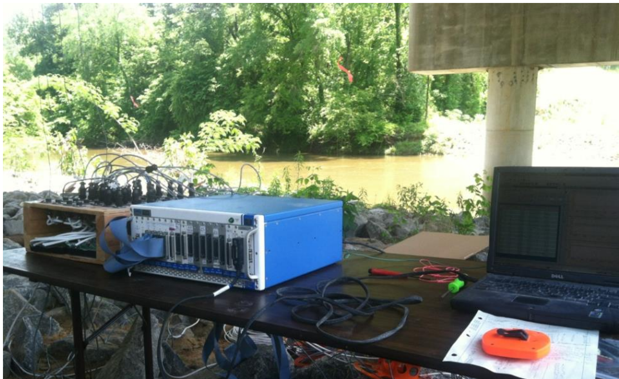
Figure 3.39. Optim Megadac® data acquisition system and sensor input channel.
