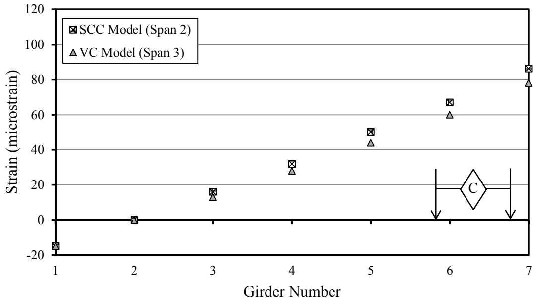
Figure E-21. Strain results from load-truck-position C on spans with BT-72 girders.
