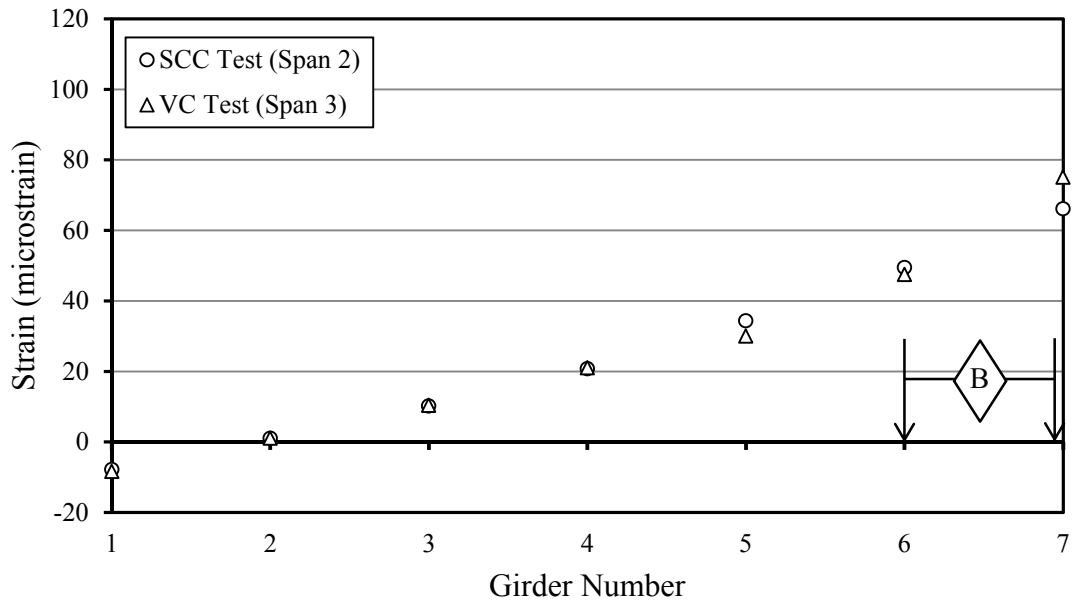
Figure A-19. Strain results from load-truck-position B on spans with BT-72 girders.
