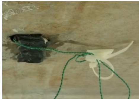
Figure 3.26. Mastic tape applied over the strain gauge for mechanical protection.
