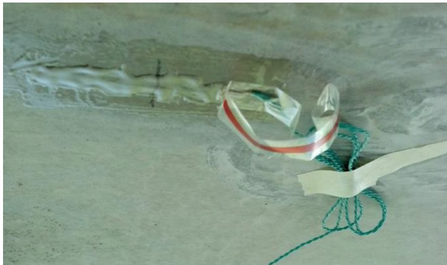
Figure 3.24. A gauge temporarily peeled back to allow for a thin layer of epoxy.
