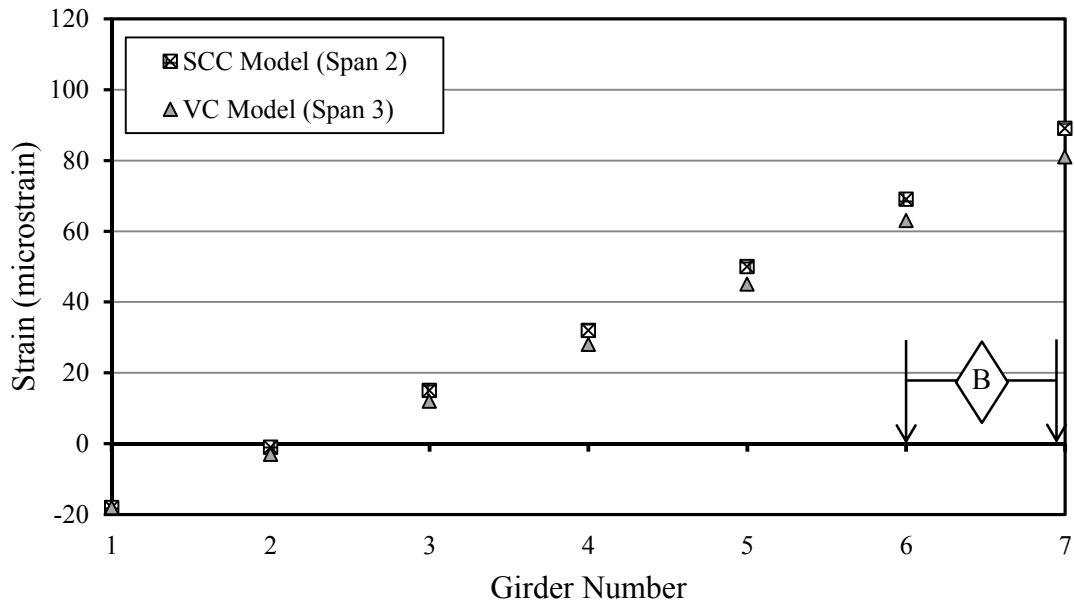
Figure E-19. Strain results from load-truck-position B on spans with BT-72 girders.
