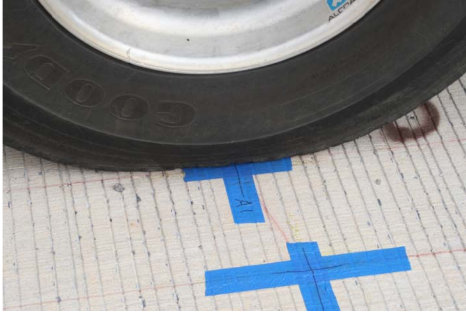
Figure 4.8. Tire positioning marks on the bridge deck.
