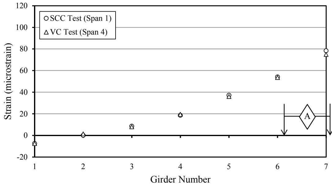
Figure A-1. Strain results from load-truck-position A on spans with BT-54 girders.
