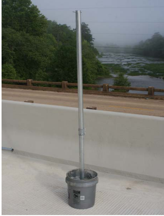
Figure 3.31. Deflectometer anchoring pole for span 3 over Hillabee Creek.
