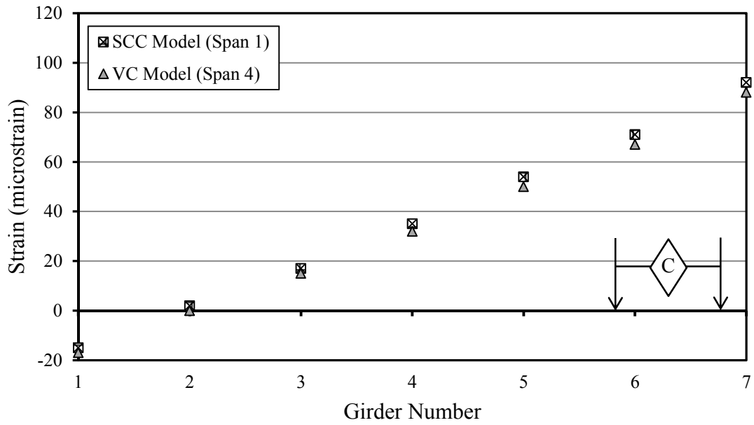
Figure E-5. Strain results from load-truck-position C on spans with BT-54 girders.
