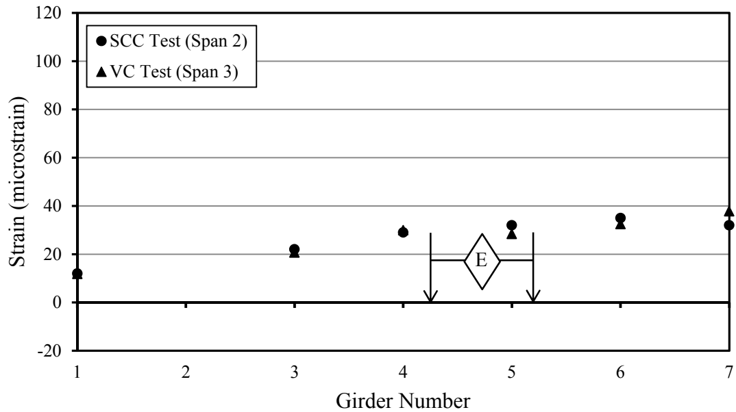
Figure B-11. Strain results from load-truck-position E on spans with BT-72 girders.
