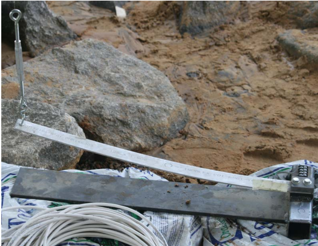
Figure 3.29. A deflectometer positioned at ground level.
