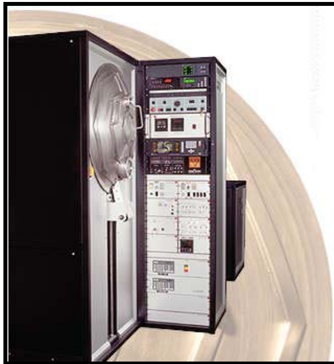
Figure 4.2 CHA- Mark 50 high vacuum deposition system used for depositing boron thin films [93].
