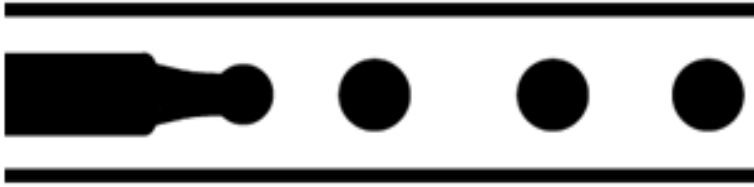
Figure 1.13 Representation of Co-Flow droplet formation with black circles representing aqueous phase.
