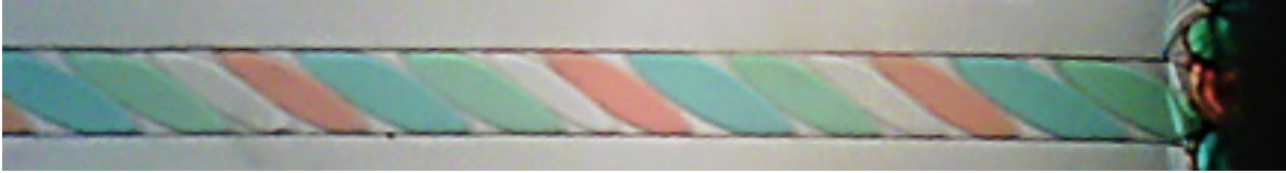
Figure 6.3 Image of droplets output from a 4 aqueous channel alternating droplet chip as it maintains the same repeating pattern in a spontaneous, passively-operated manner.
