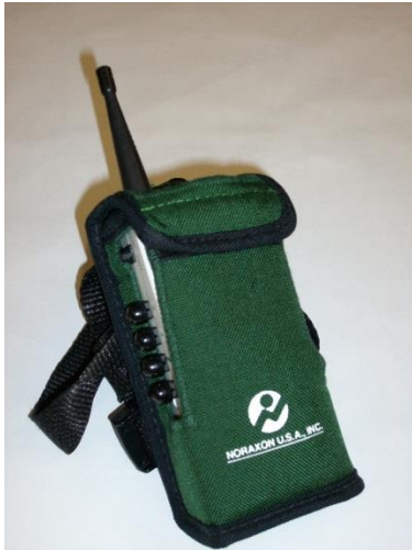
Figure 11. Noraxon Telemetry 2400T V2 wireless transmitter.
