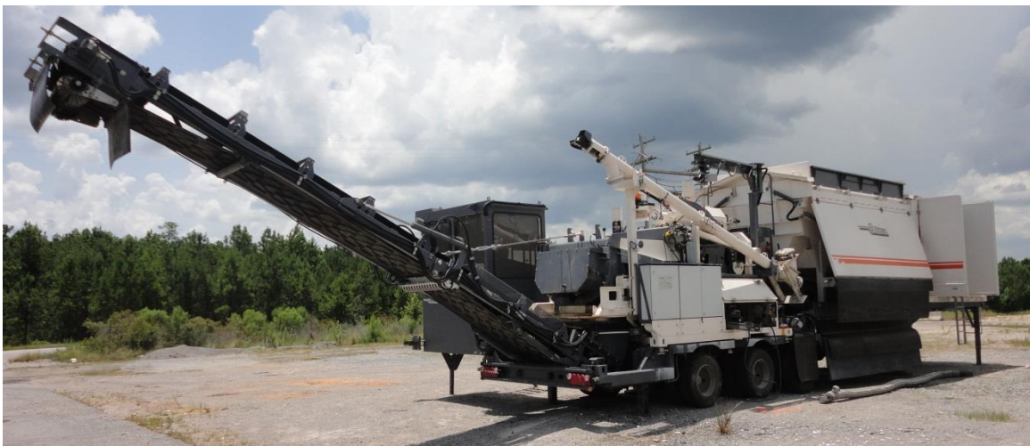
FIGURE 3.7 Mobile Cold-Recycling Plant used at the NCAT Test Track
