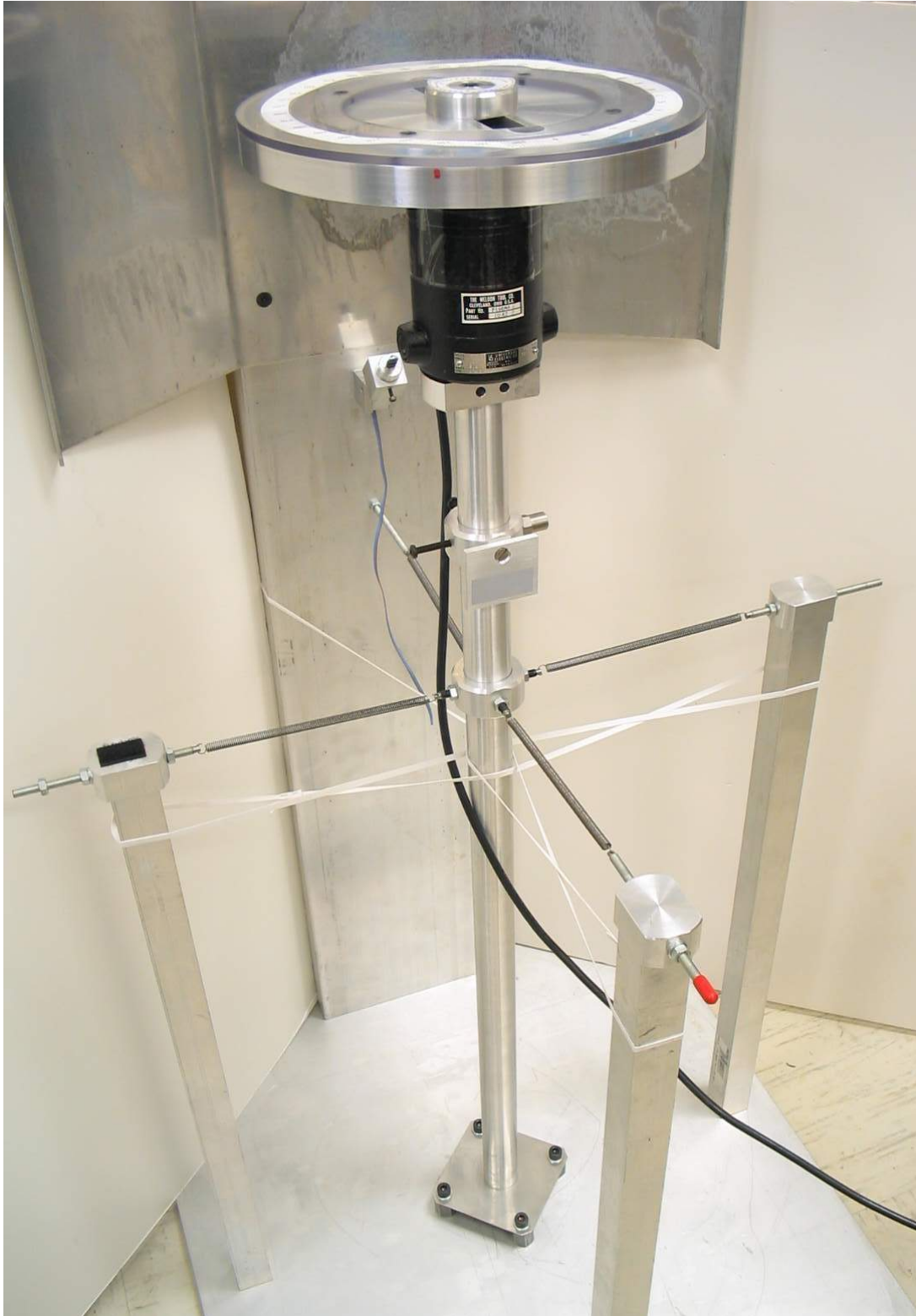
Figure 3.25 Side view of ball balancer experimental facility
