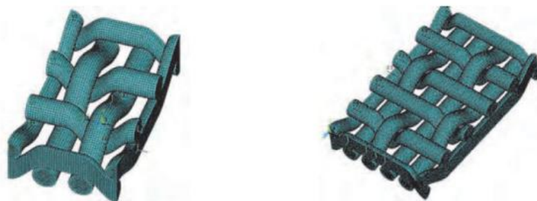
Figure 8 Solid FE model of unit cell of twill (left) and satin (right) woven structure [48]
