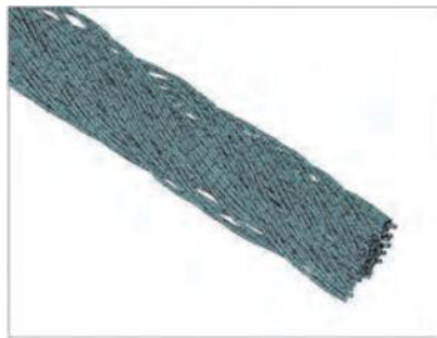
Figure 6 Beam model of filaments for loose structure [43]
