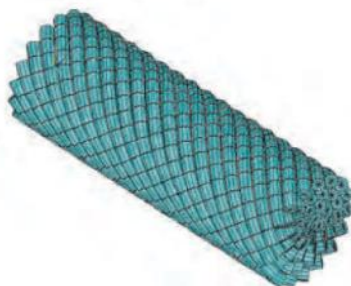
Figure 7 Beam FE model of 50-filament twisted yarn [43]
