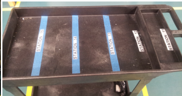
Figure 4.15: Push cart for material delivery
