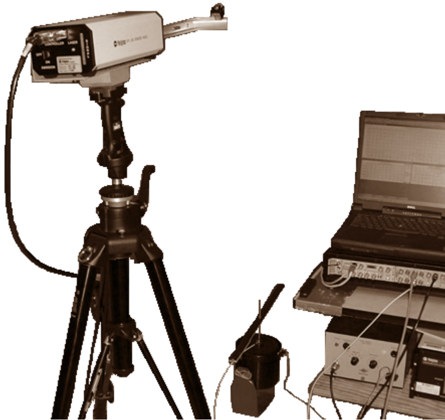
Figure 3.5. Experimental setup for damping measurements.
