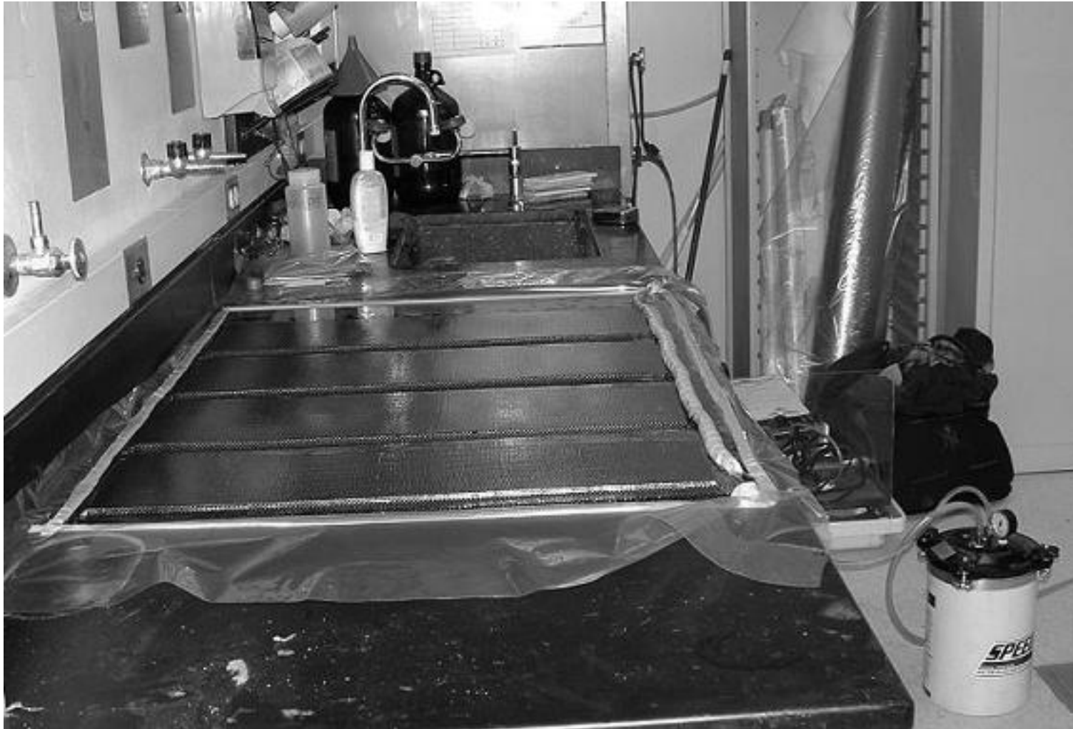
Figure 1.2. Fabrication of foam-filled honeycomb sandwich panels.
