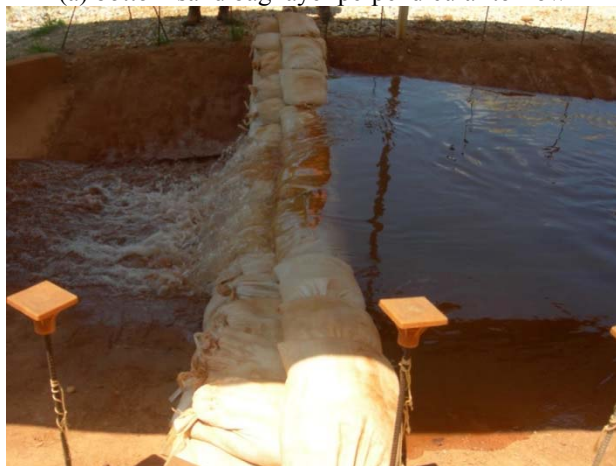
(c) top sand bag layer perpendicular to flow
