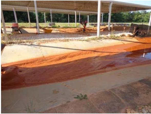
(e) large particle sediment deposition near channel head
