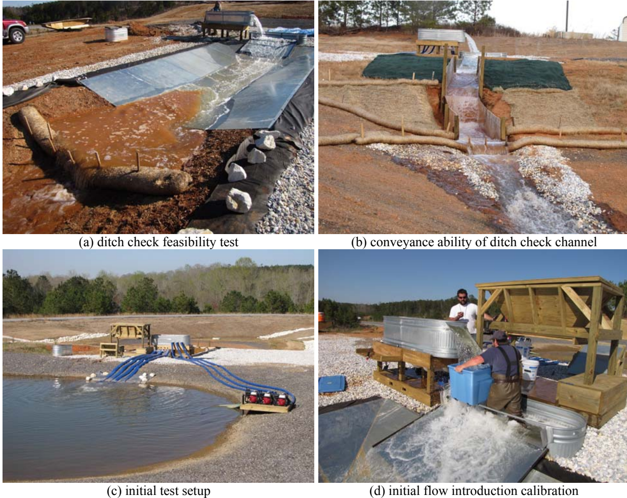
Figure 4.20: Initial Testing to Evaluate Ditch Check Channel Testing Feasibility.
