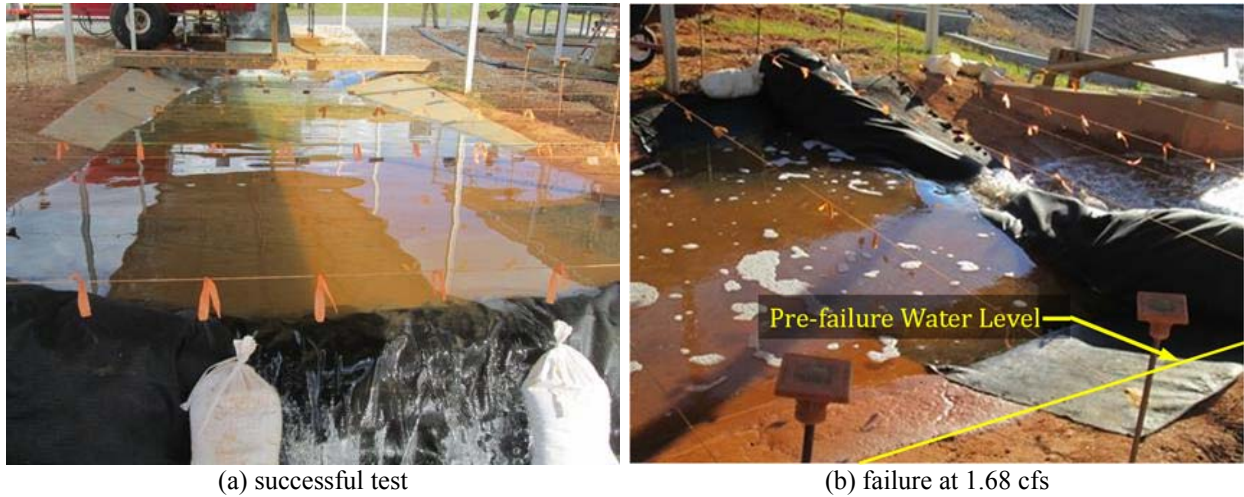
Figure 6.25: Sand Bag Burrito Ditch Check Test.
