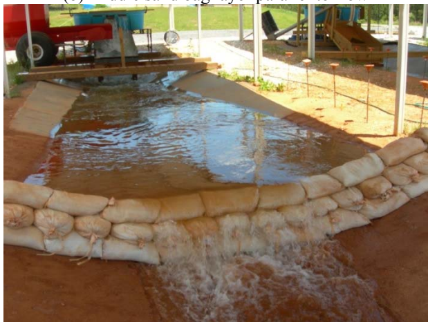
(d) test during third flow tier of 1.68 cfs
