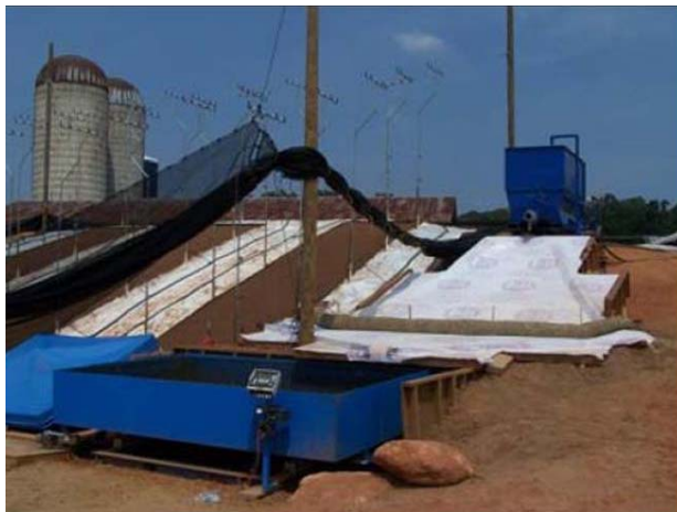
(a) sheet flow intercept pretest setup
