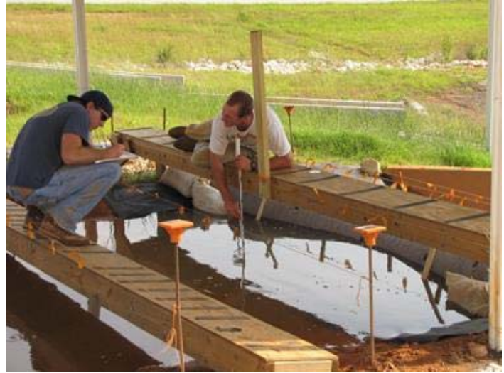
(b) depth and velocity measurements during testing
