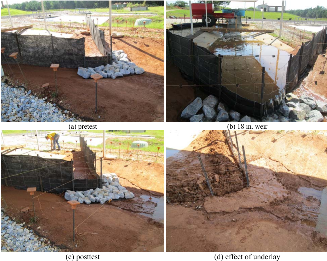
Figure 6.18: TnDOT Enhanced Silt Fence Ditch Check Test.
