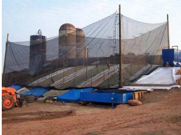
Figure 2.8: TRI's ASTM D 6459 Setup (TRI 2008).
