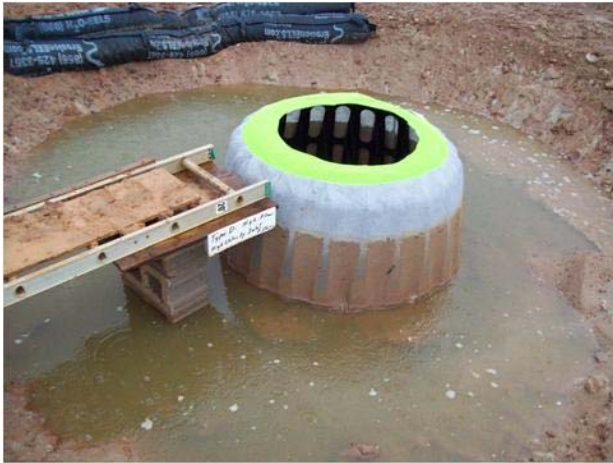
(a) drop inlet test
