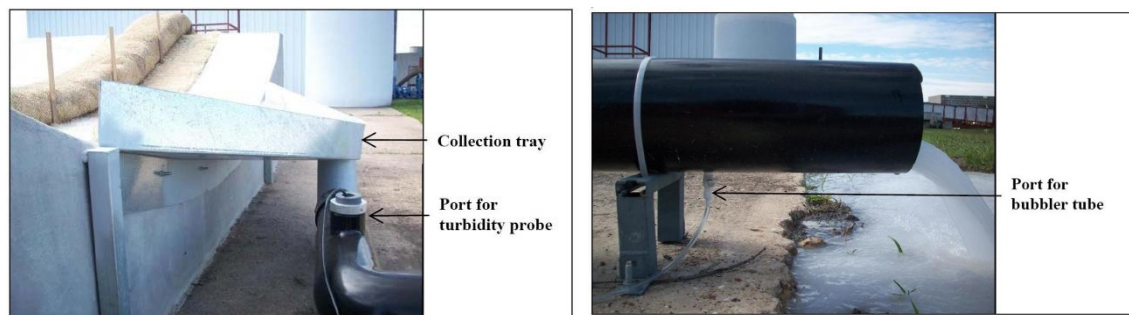
(a) flume collection system (b) sediment-laden water discharge system Figure 2.2: TTI Sediment Collection and Discharge System (McFalls et al. 2010).
