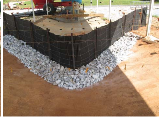
(b) modified no. 4 dissipater pretest
