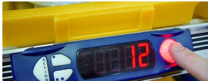
Figure 3.8: A Representation of the Pick to Light Systems
