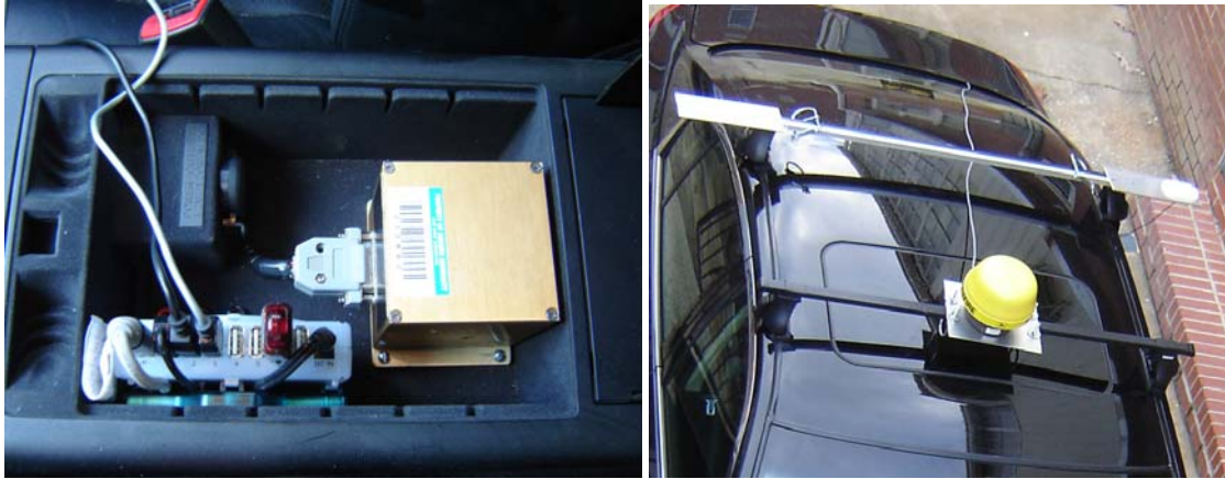
Figure B.2: The Crossbow IMU (left); Starfire and Beeline (right).
