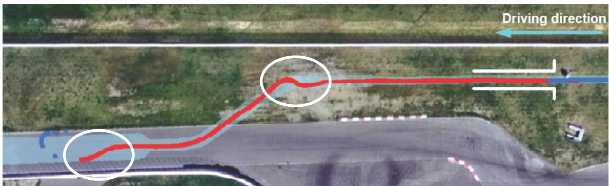
Figure 2.9: Dead reckoning after a 200 foot tunnel at the NQE.
