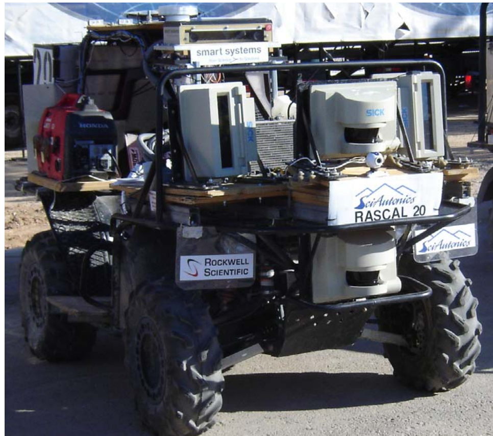
Figure A.4: Obstacle detection sensors on RASCAL.
