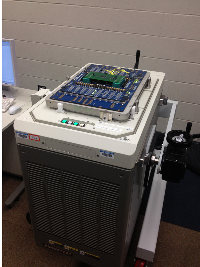
Figure 2.3: Test head of the Advantest T2000GS with an FPGA on the loadboard.
