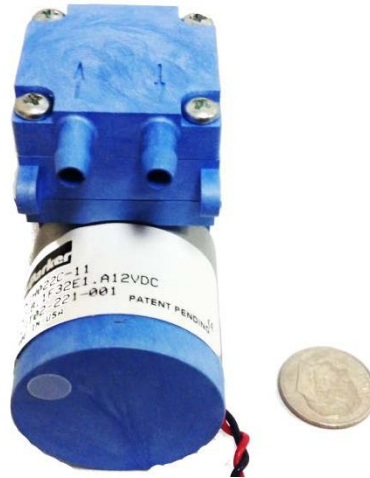
Figure 19: Parker Fluidics H022C-11 diaphragm pump used to provide gas to the E2V IR11EJ while conducting micropump experiments with a dime shown for size comparison.
