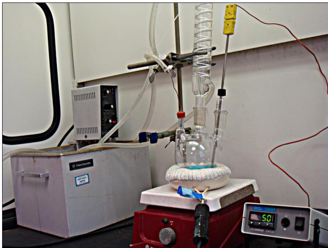
Figure 3.2 The reaction set-up for the high-temperature synthesis of Co nanoparticle clusters.
