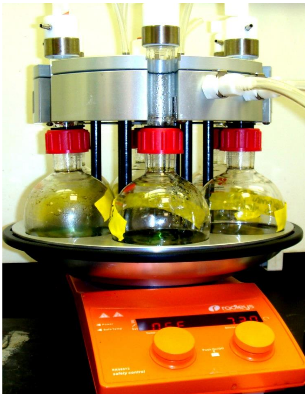
Figure 4.1 Radley apparatus used to simultaneously synthesize up to six Co nanoparticle samples in DMSO.
