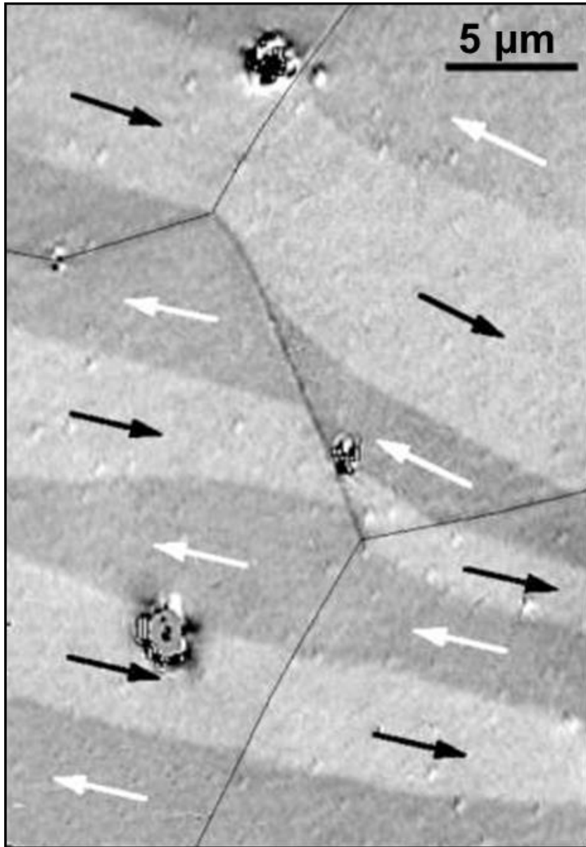
Figure 1.4 An image of a neodymium magnet obtained using Kerr microscopy (Hubert & Schafer 2000).
