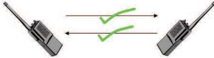
Figure 1.6: Full-duplex wireless transmission
