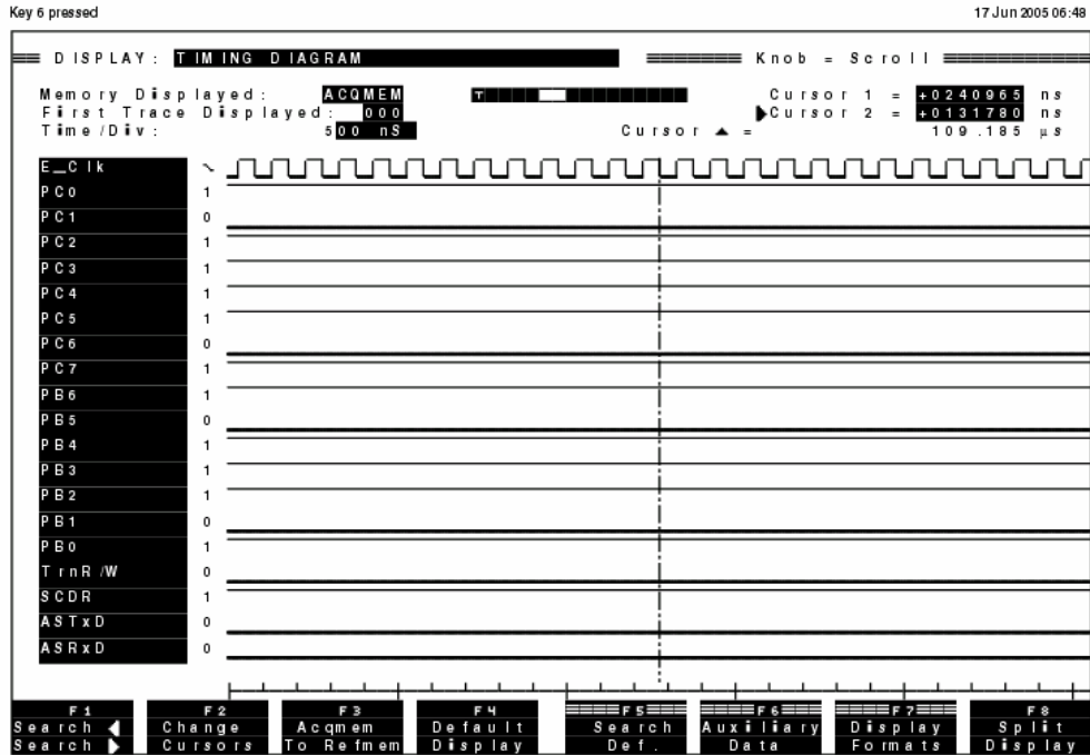
Figure 4.2- Key 6 is pressed (10111101=>row 2 and column 3 are shorted)
