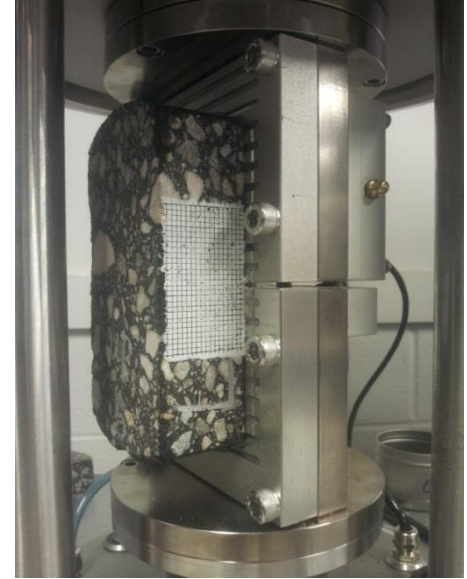
Figure 3.7 Setup of specimen glued on base plates in AMPT
