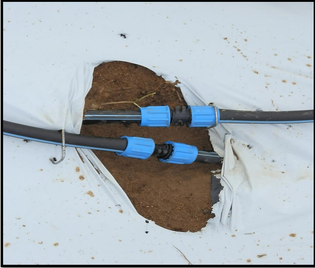
Figure 2. Herbicide treatments were delivered to polyethylene-mulched beds by splicing main delivery lines (1.27 cm plastic tubing) into the drip tape using drip tape connectors.
