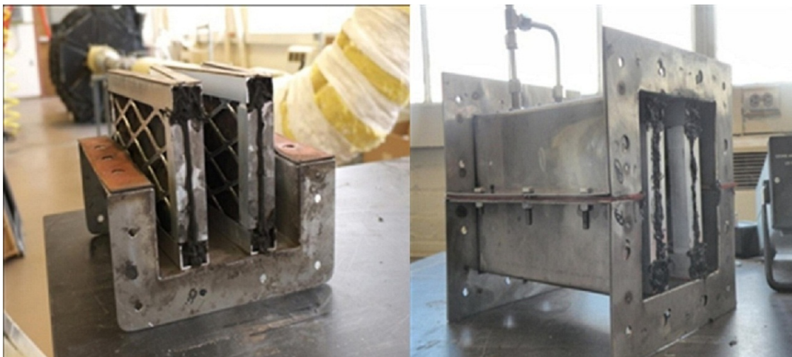
Figure II.6: MFEC VOC converter (W-shaped structure)
