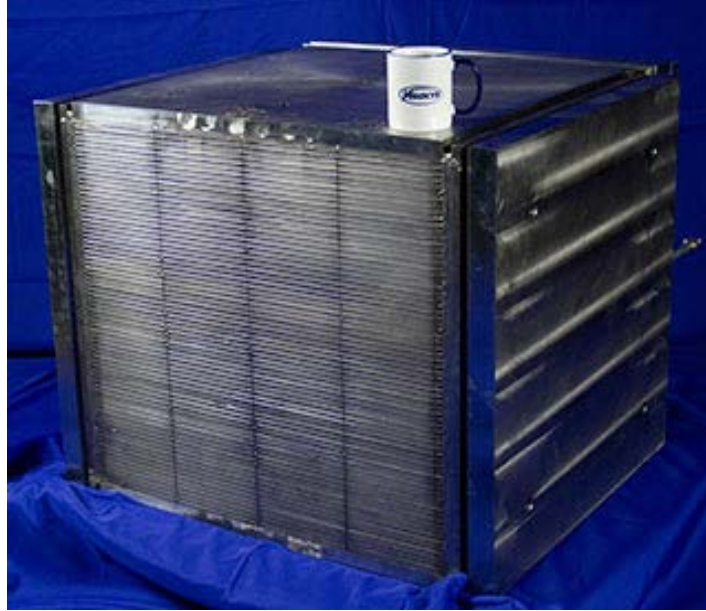
Figure I.7: A microchannel reactor (reproduced from www.hatch.com.au/News_Publications/Energy_Innovation )
