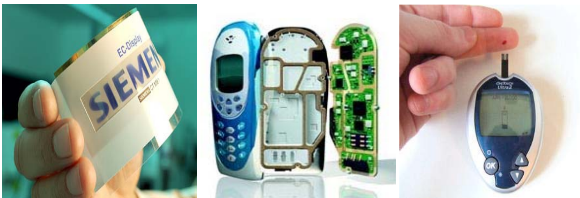
Figure 1. Different applications of CPs in; a) an electrochromic display, b) an electromagnetic shielding component, c) a glucose sensor
