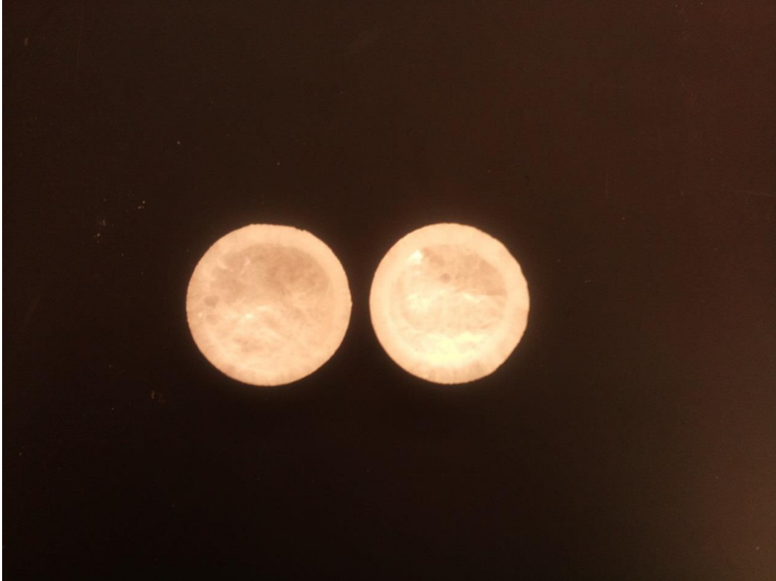
Figure 3-15: N-Hexacosane (C 26 H 54 ) solid samples obtained following the oven solidification process (approximately diameter of 2.5 cm and thickness of 1 cm) (sides shown in the figure were exposed to the atmosphere)
