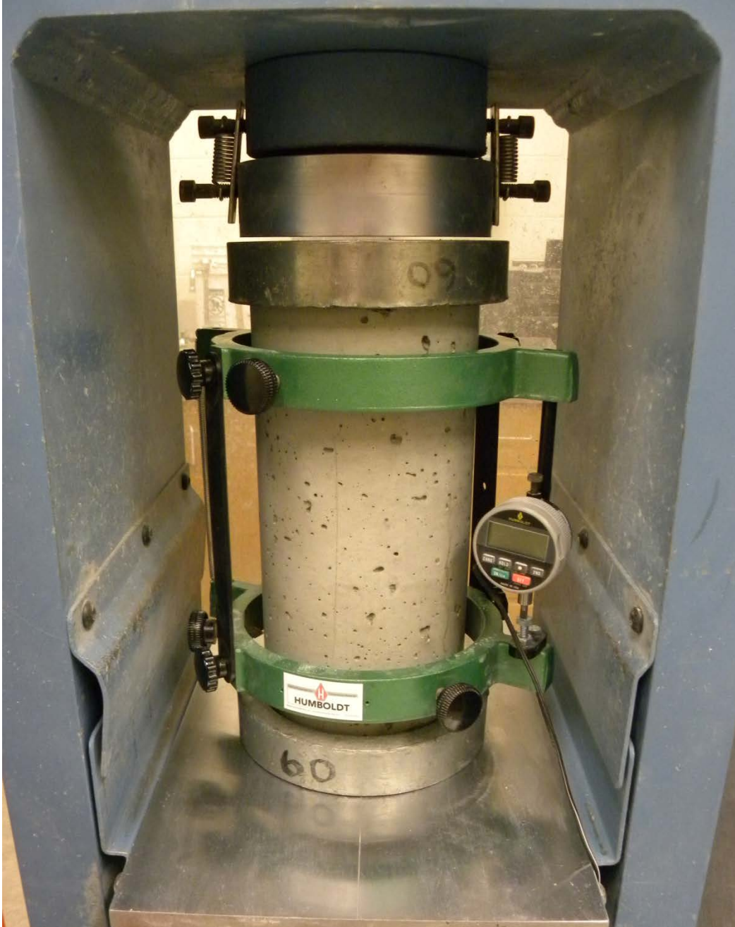
Figure 4.17: Cylinder Ready for Modulus Testing
