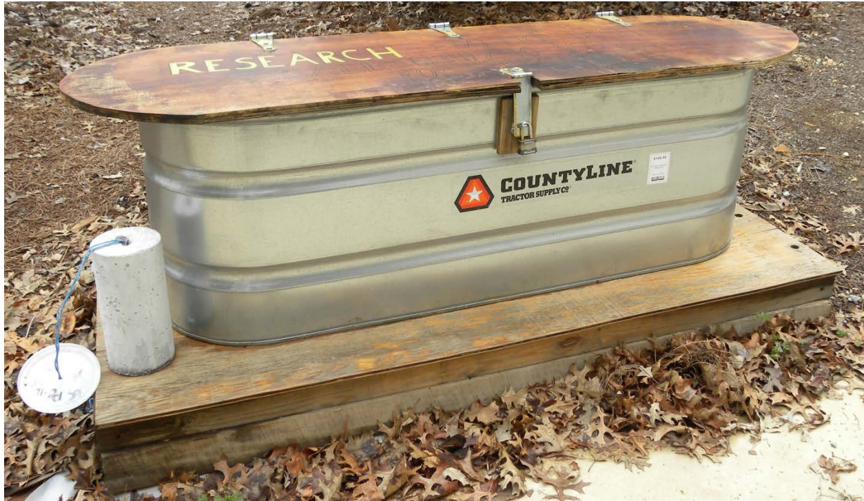
Figure 4.13: Curing Tank Used for Field-Cure Cylinders
