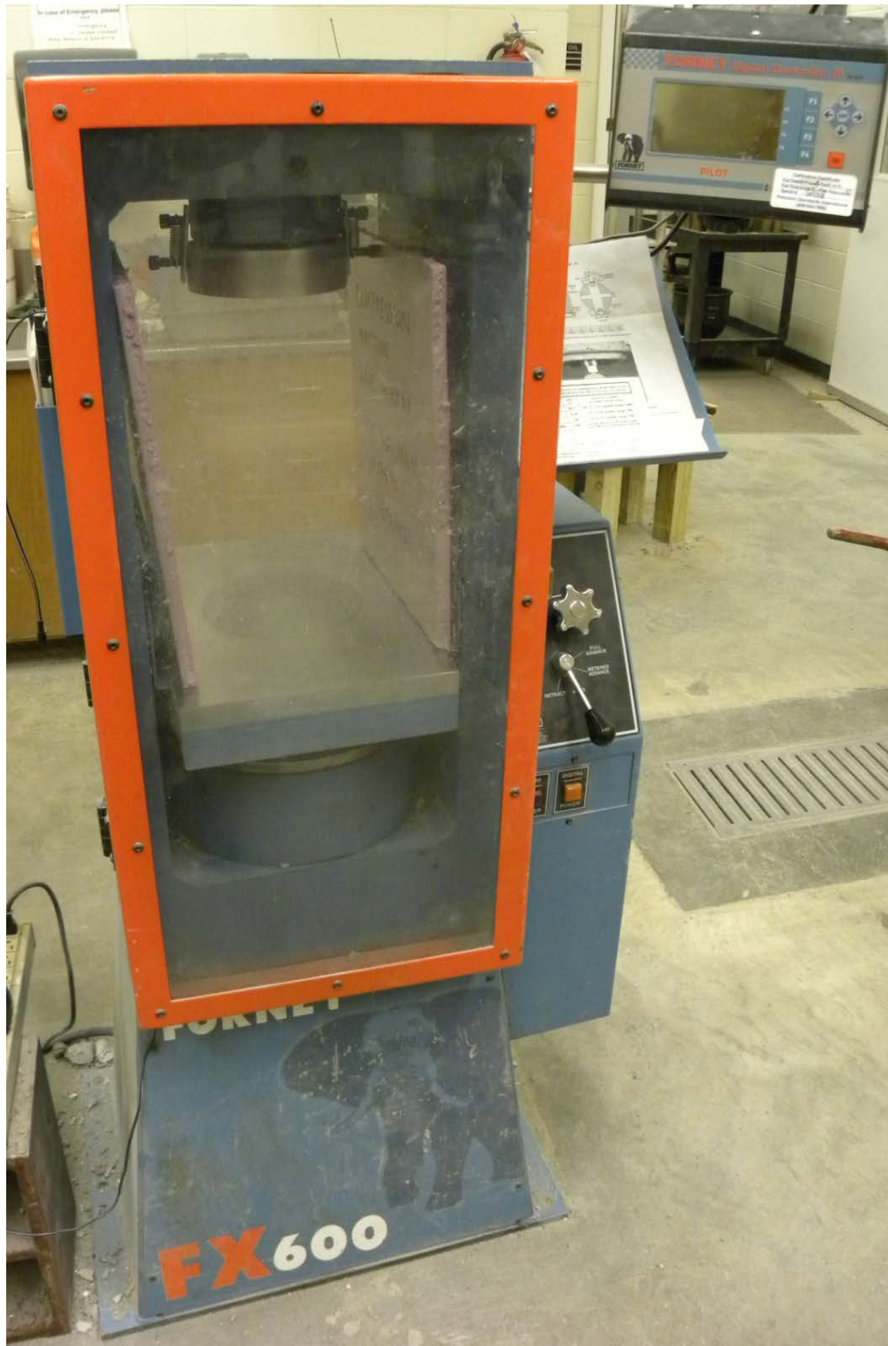
Figure 4.15: Forney FX600 Compression Machine Used for Testing
