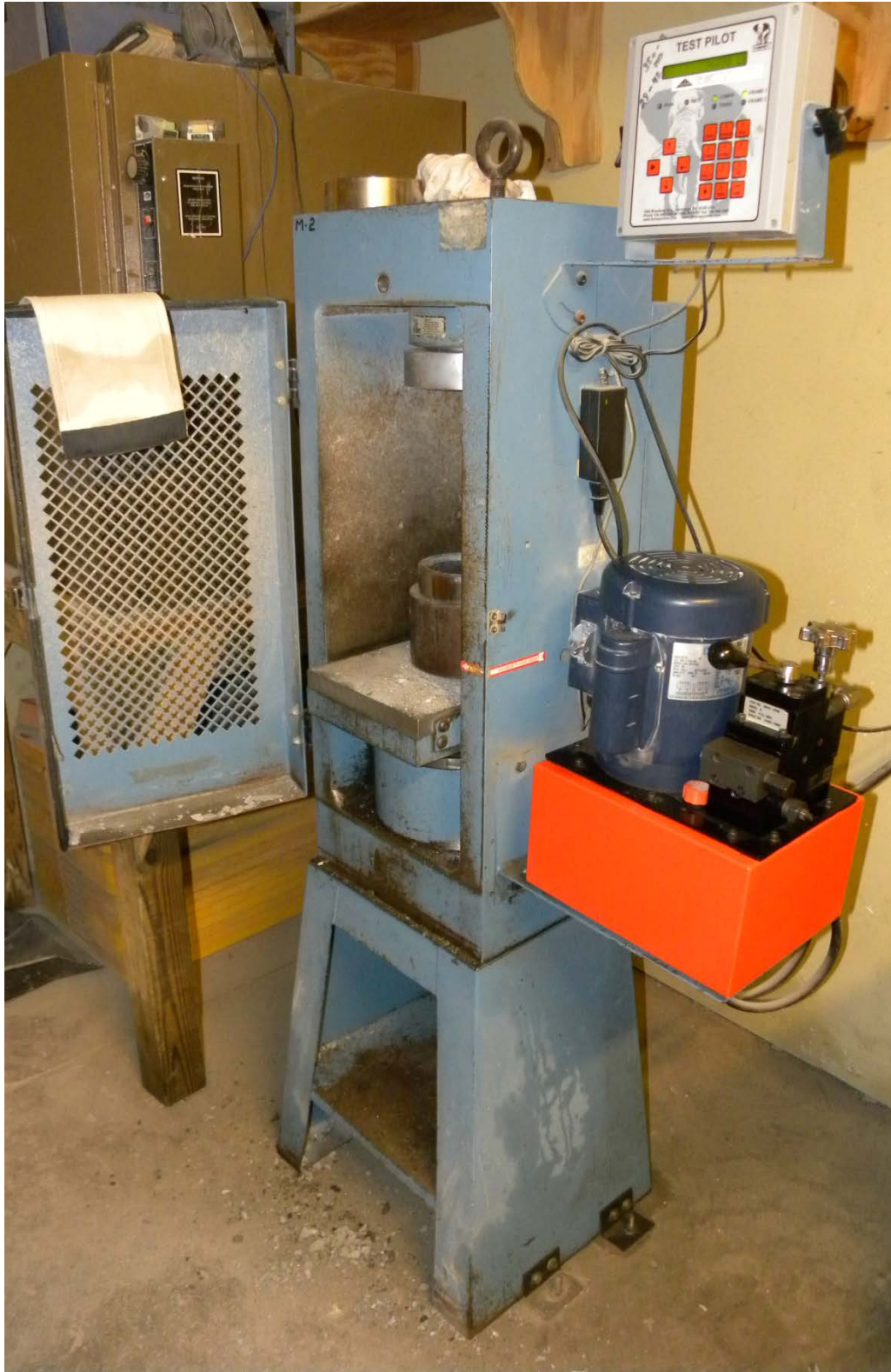
Figure 3.16: Compression Testing Machine from Plant D
