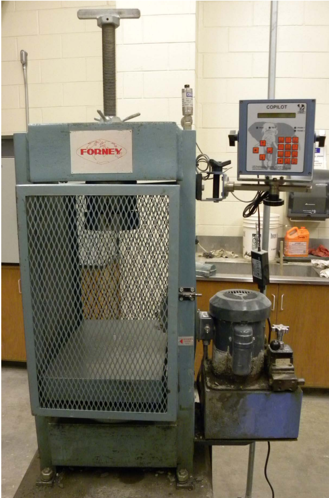
Figure 4.16: Forney QC400 Compression Machine Used for Testing
