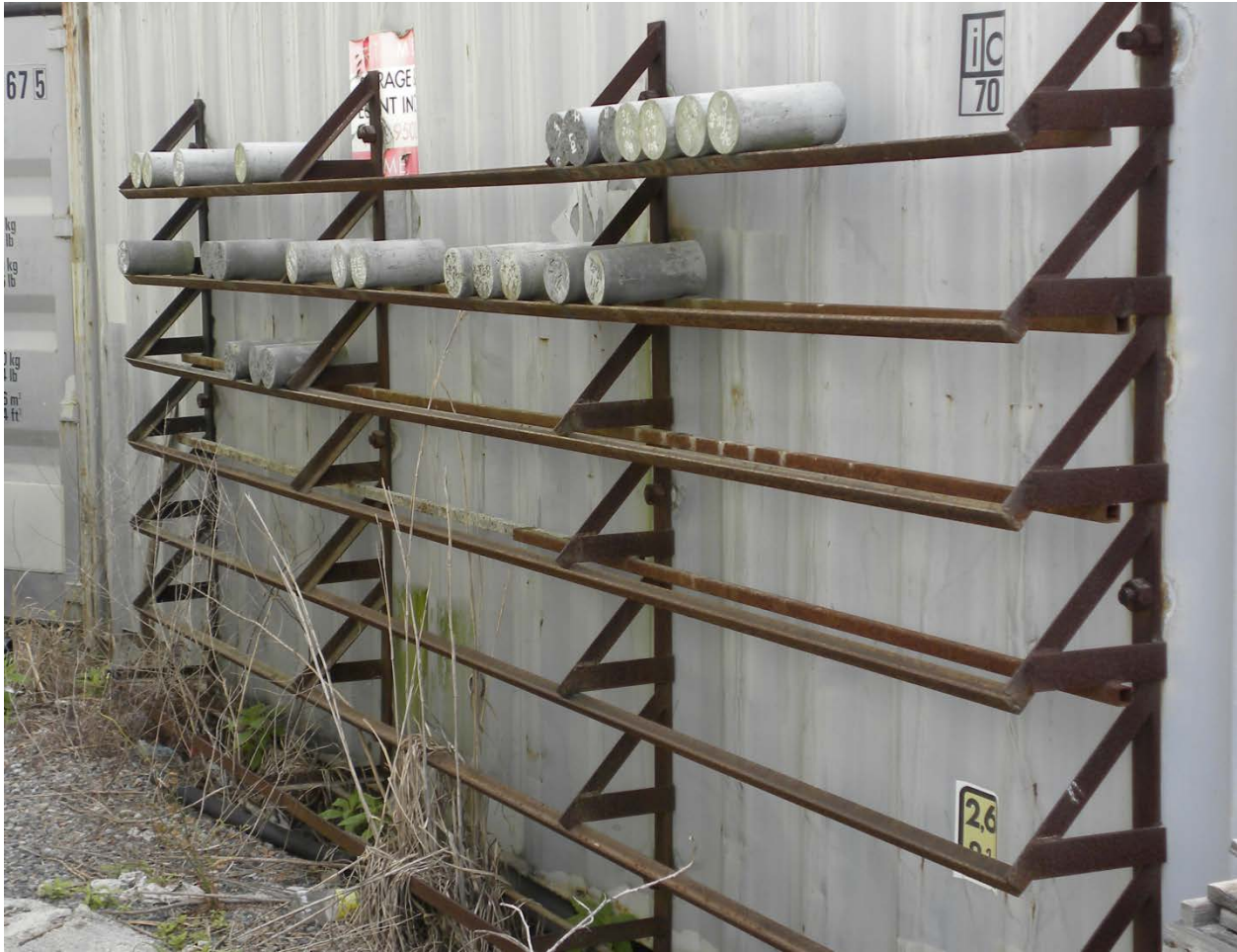
Figure 3.20: Curing Racks Used for Cylinders at Plant D
