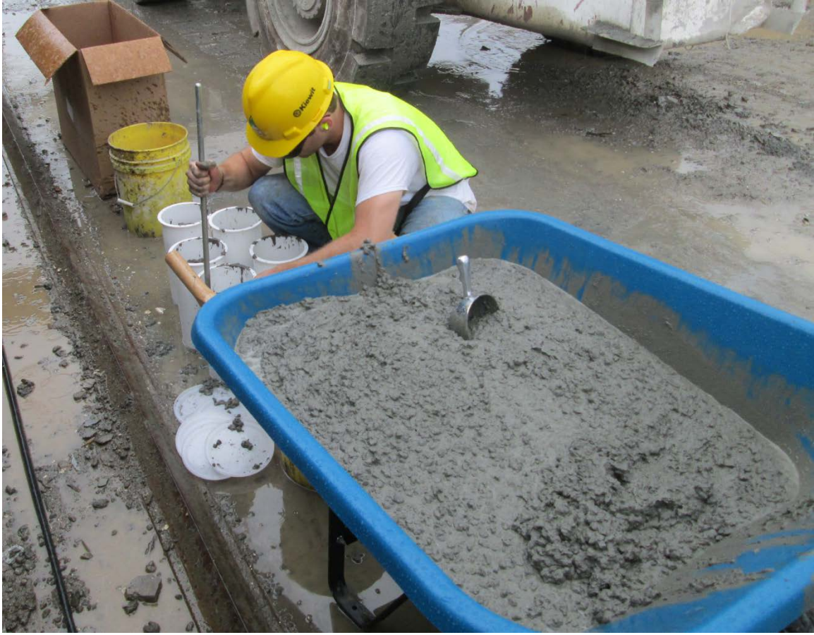
Figure 4.6: AUHRC Researcher Producing Test Cylinders
