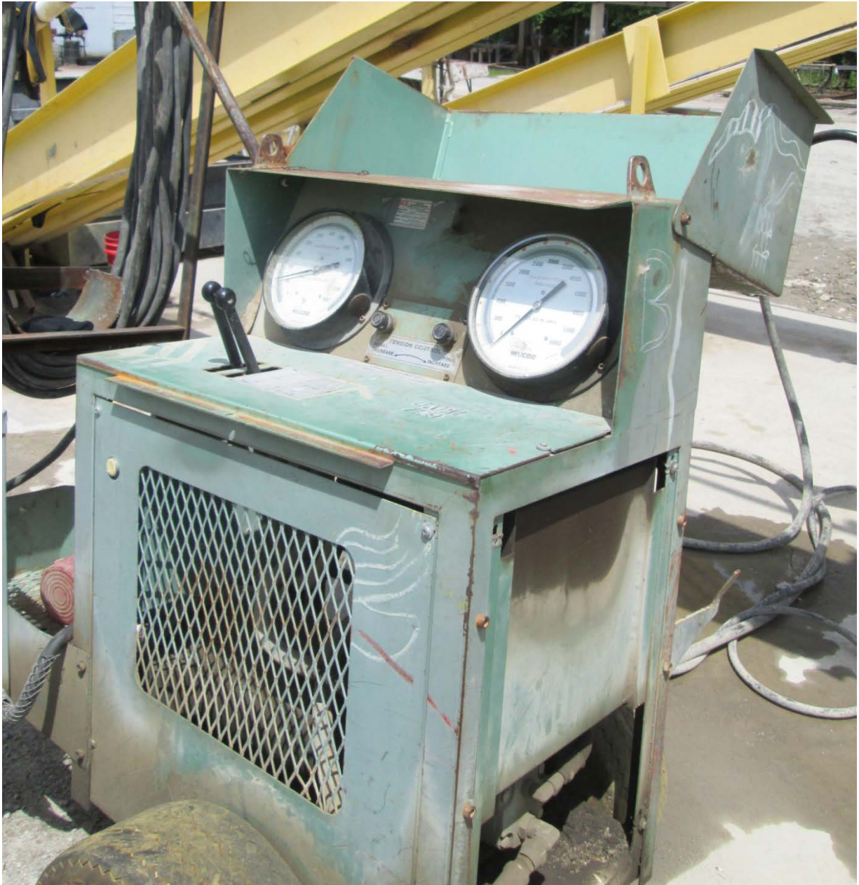
Figure 3.6: An Example Strand Tensioning Machine from Plant B
