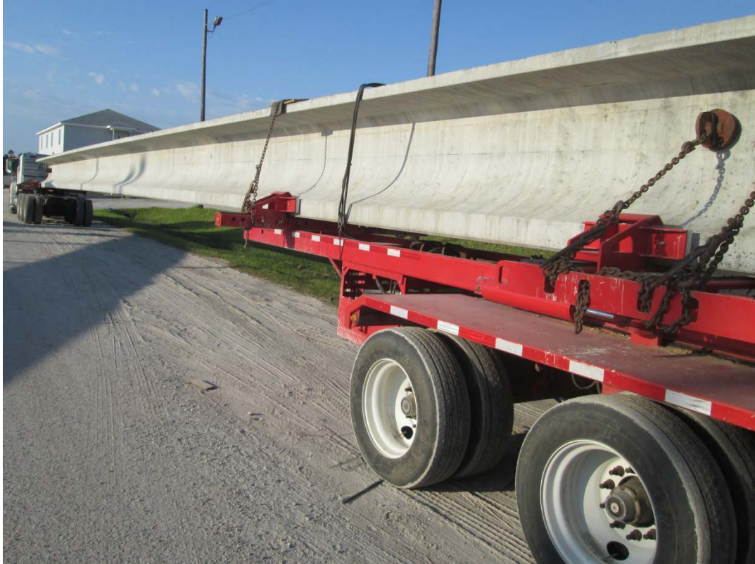
Figure 3.30: A Girder Being Transported by a Split-Bed Trailer
