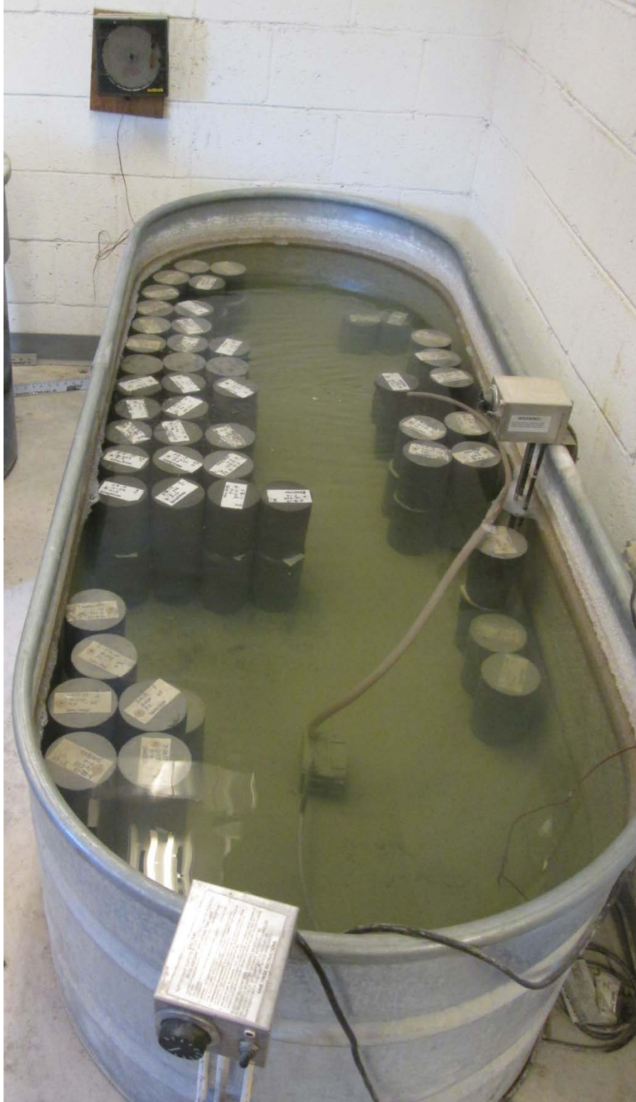
Figure 4.12: Temperature-Controlled Lime Bath Used for Standard-Cure Cylinders
