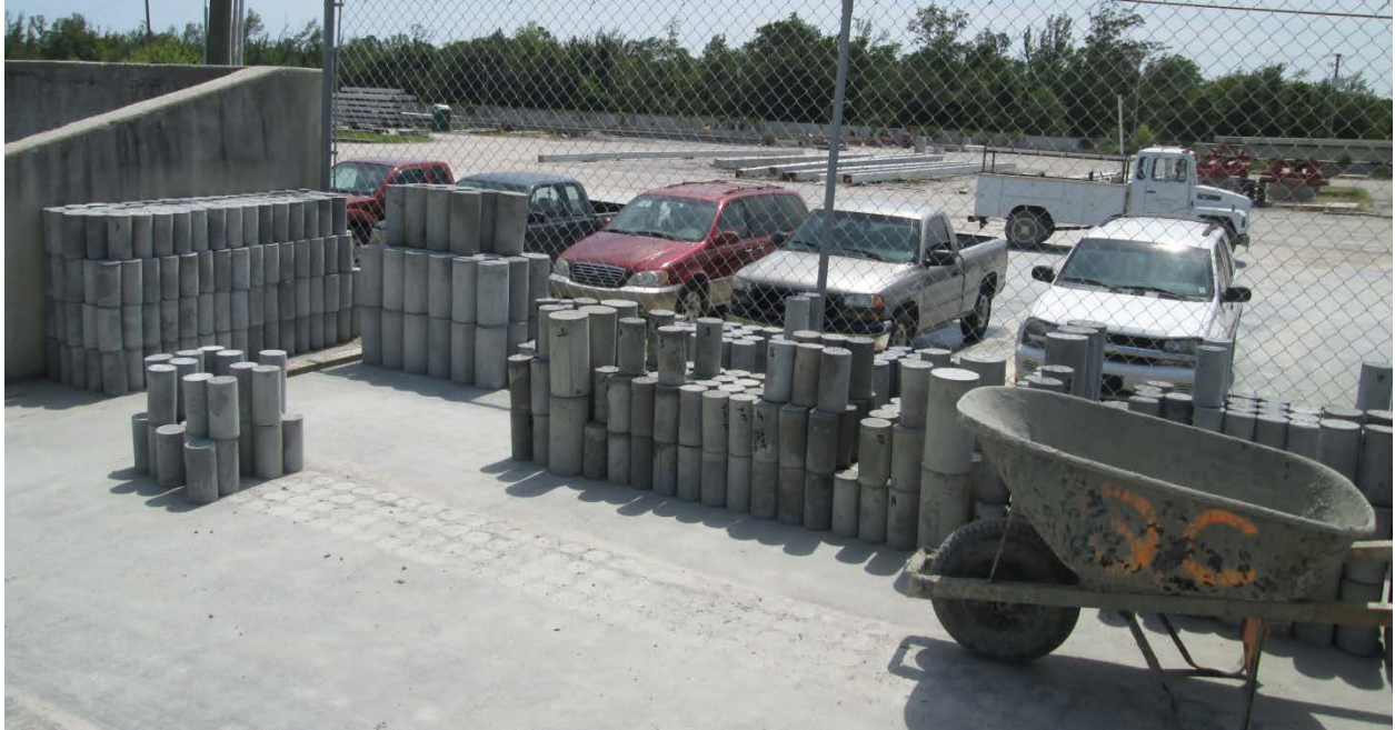
Figure 3.19: Curing/Storage Conditions for Cylinders at Plant C
