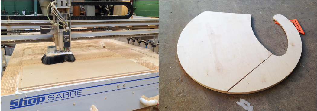
Figure 6.32: Board Cutting by CNC Router Machine
