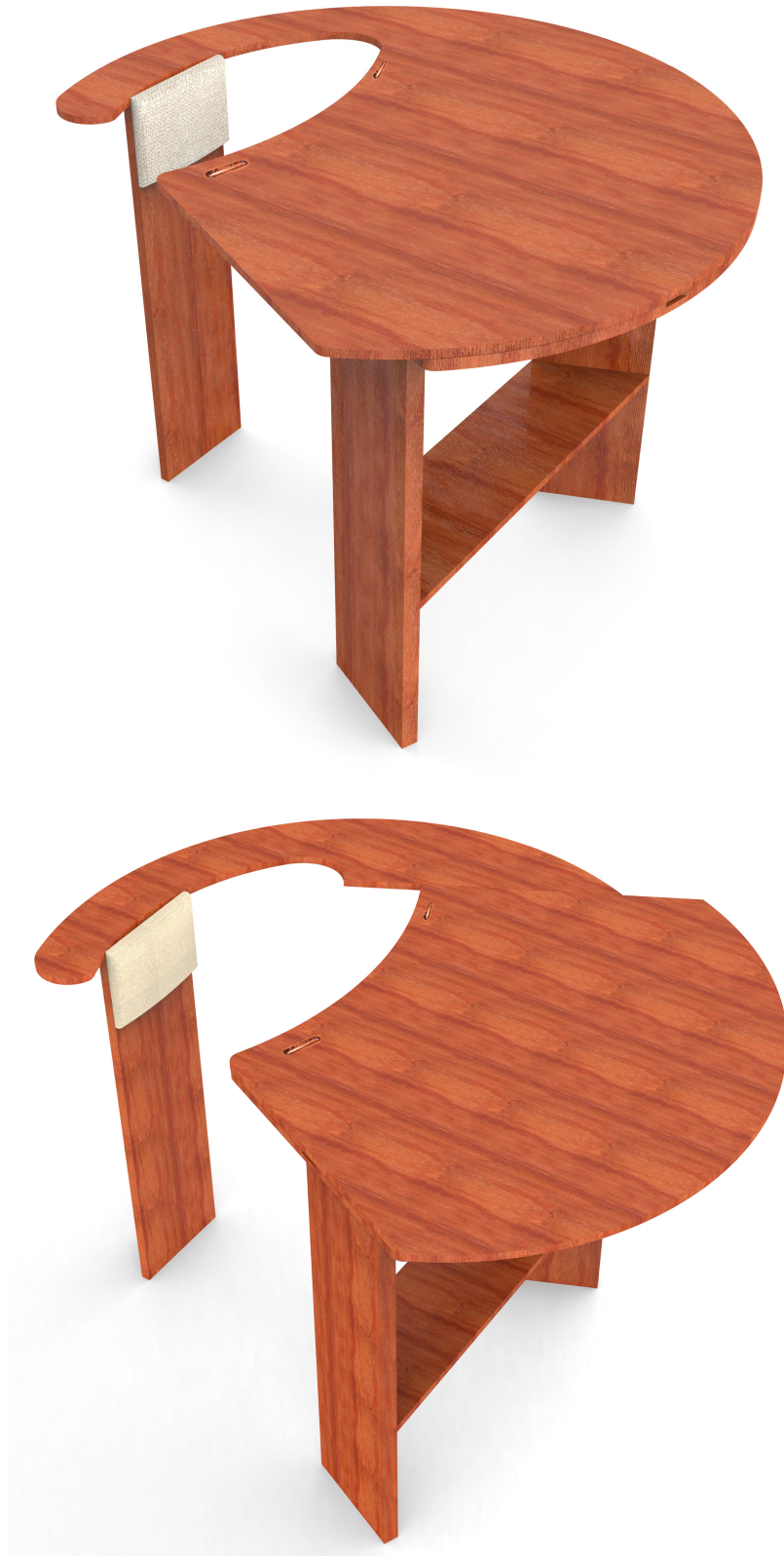
Figure 6.27: Top Board Opening and Closing Status in Perspective View
