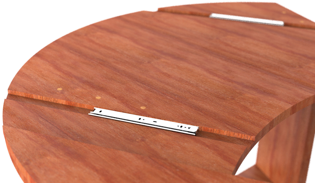
Figure 6.30: Design Details around Drawer Slides Area
