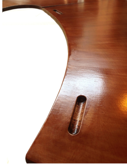
Figure 6.36: Dents for Dragging Top Board and Steel Plate for Stopping Top Board
