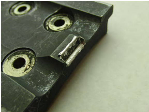
Figure 6.1: Example of wear on a mid shoe
