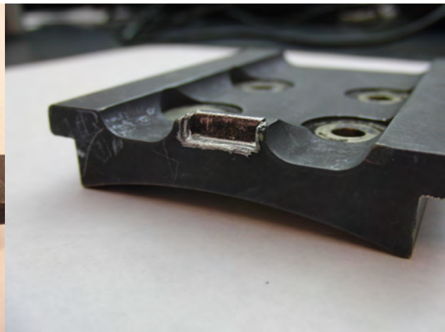
Figure 6.64: After experiment: mid shoe deformation and wear from the latch face
