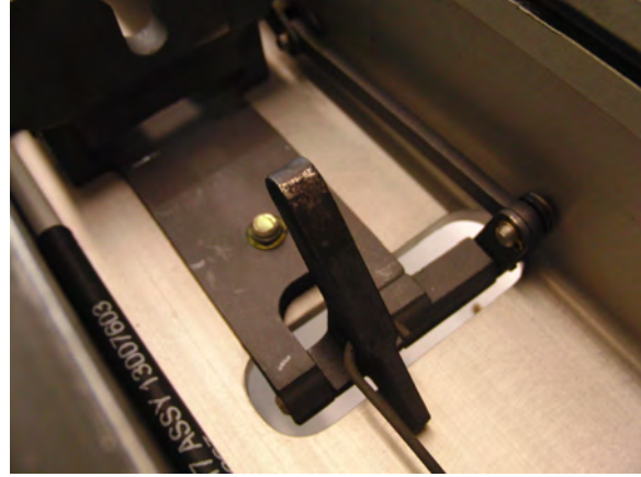
Figure 6.28: After: mickey mouse ears finger wear
