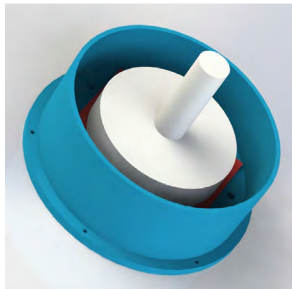
Figure 4.3: Entire persistent contact test fixture
