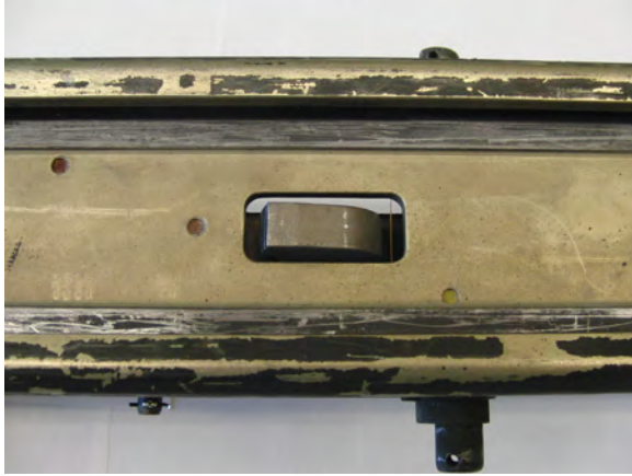
Figure 6.9: Latch from the rail face
