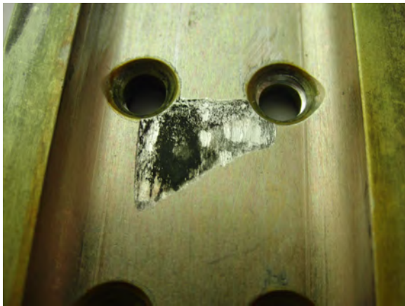
Figure 6.23: After: rear shoe wear from leaf spring
