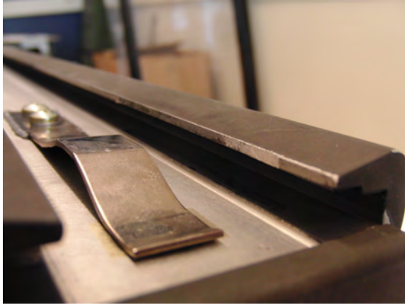
Figure 6.25: After: rail edge wear from rear shoe
