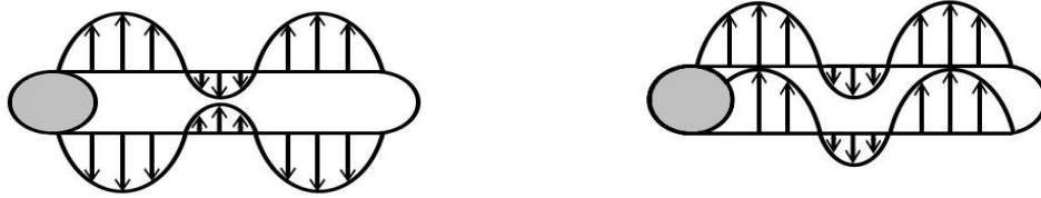
Figure 9: Cylinder with active control, left showing the in-phase mode and right showing the out-phase mode
