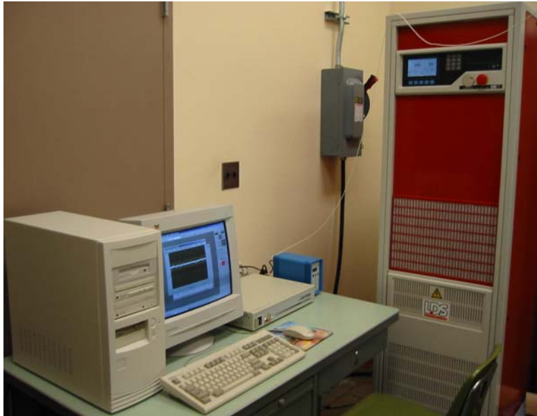
Figure 3-8 DACTRON vibration control system and SPAK amplifier
