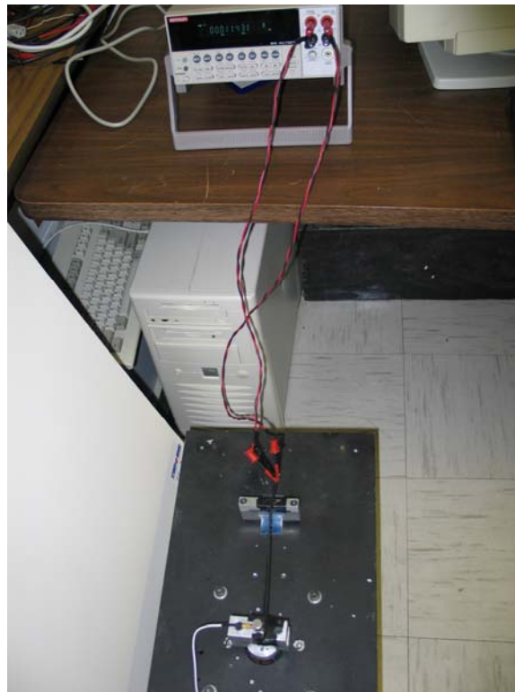
Figure 4-6 Method 2: resistance measurement in the electromagnetic interference test
