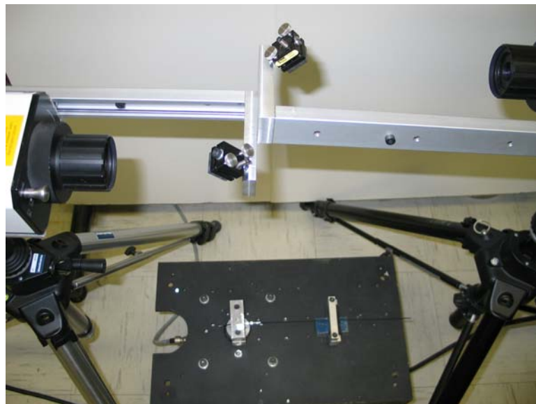
Figure 4-10 Transfer function measurement for the blade/receptacle pair
