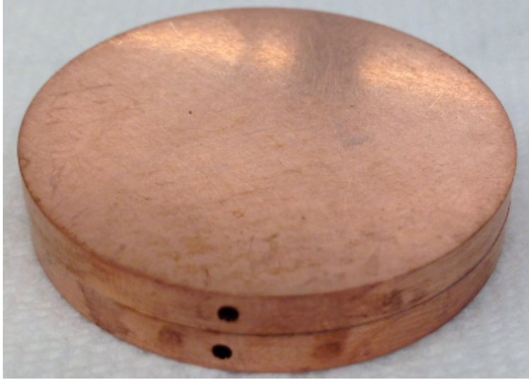
Figure 4.3: Alloy 110 Copper Disks
