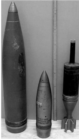
Figure 4.11: UXO items from left to right 155mm, 105mm, and 107mm shell
