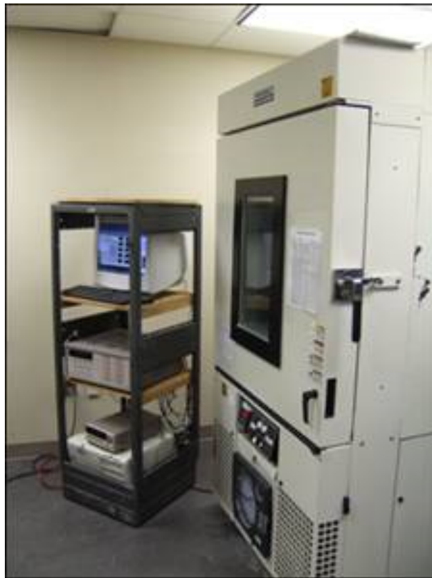
Figure 6.24: Blue M ETC-16 Environmental Chamber used for Thermal Cycling
